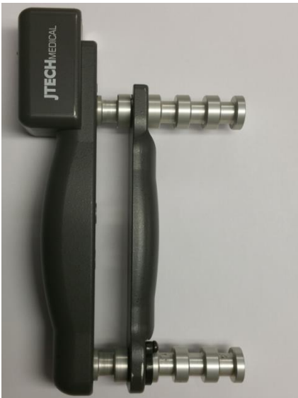
Figure 2 J-Tech computerized grip dynamometer
