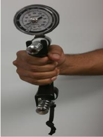
Figure 1 Jamar hydraulic grip dynamometer
