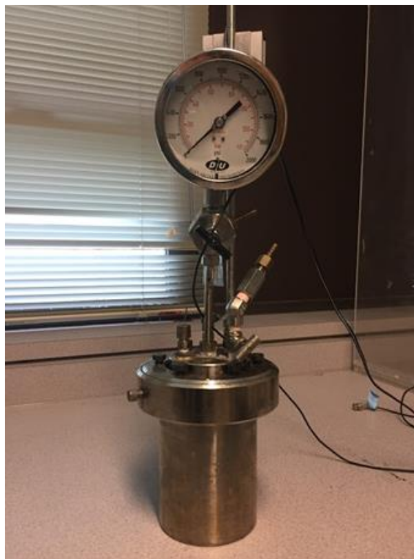
Figure 3-9: Electrochemistry autoclave used for experiments above 100 °C
