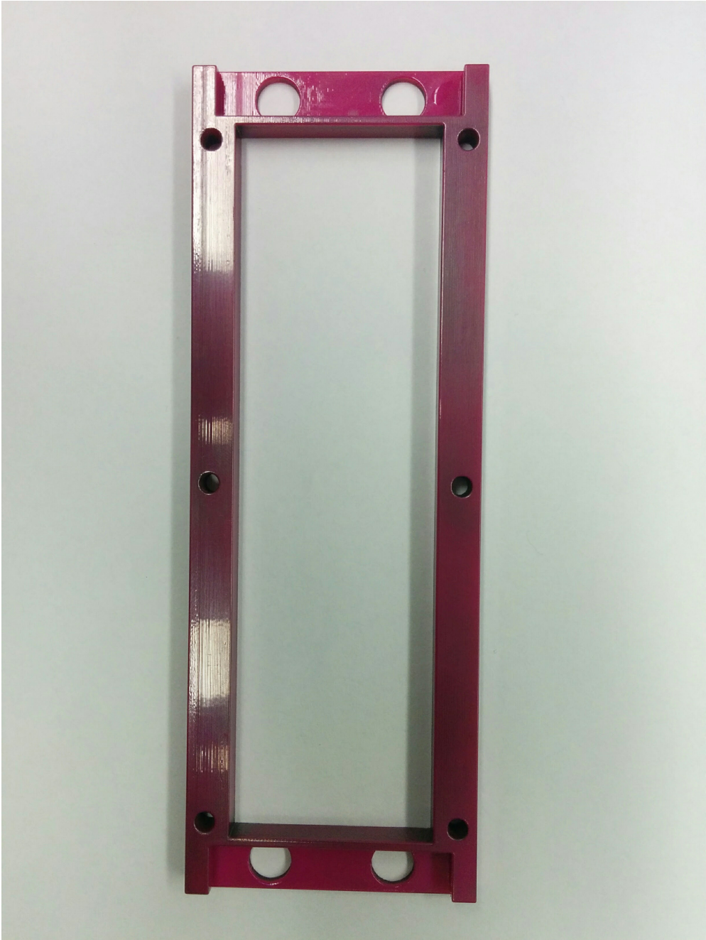
Figure 4.7: DEA mask for when the electrode is sprayed on the film.
