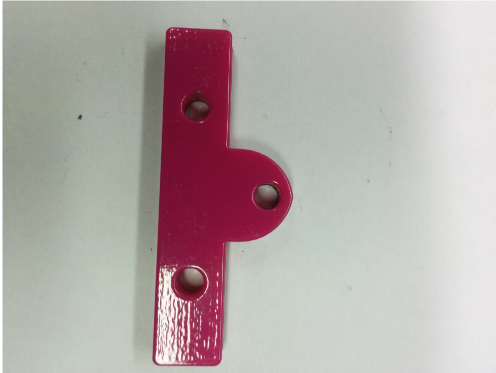
Figure 4.6: DEA end piece that is used to attach the DEA to the arm.
