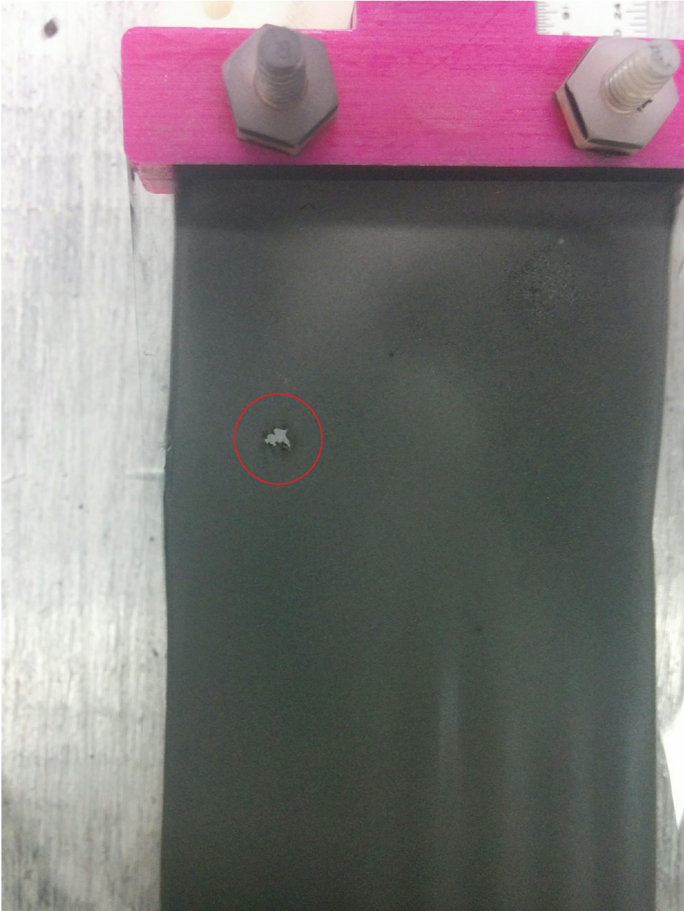
Figure 4.21: Result of dielectric breakdown in a DEA. The red circle shows the damage from dielectric breakdown.
