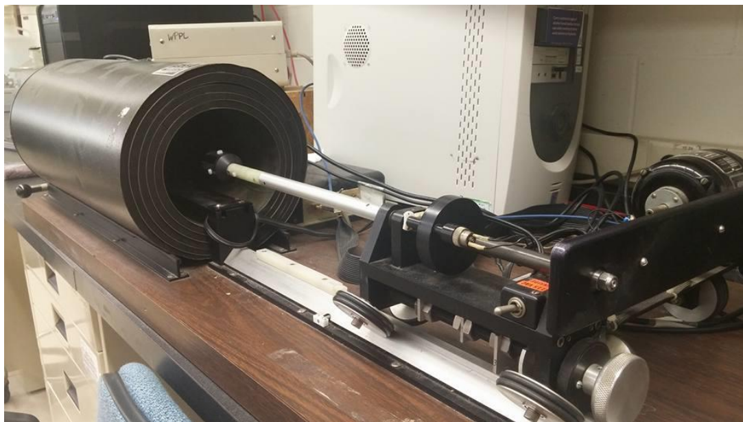
Figure 6.8 - Schonstedt SSM-2 spinner magnetometer at the Western Paleomagnetic and Petrophysical laboratory
