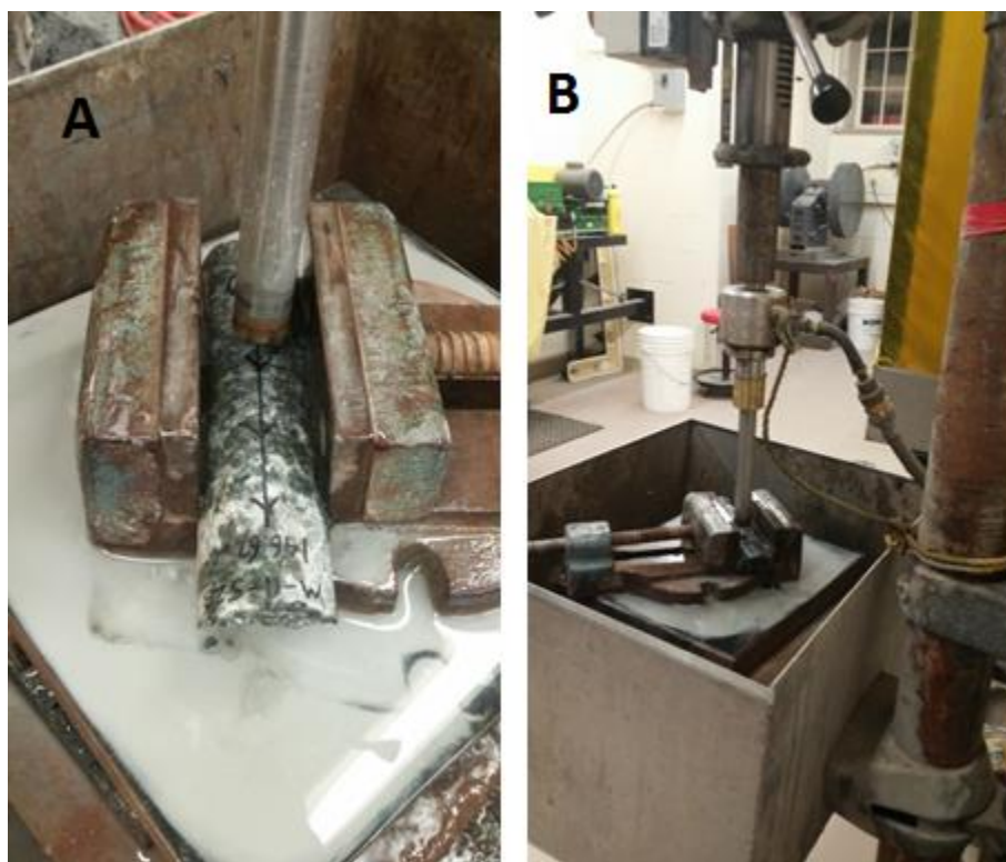
Figure 3.2- A drill press is used to obtain specimens from drill core samples. The samples are drilled perpendicular to the drill core axis as seen in A). The specimens obtained from this drilling procedure will be subjected to petrophysical assessments. A figure of the drill press is indicated by B)
