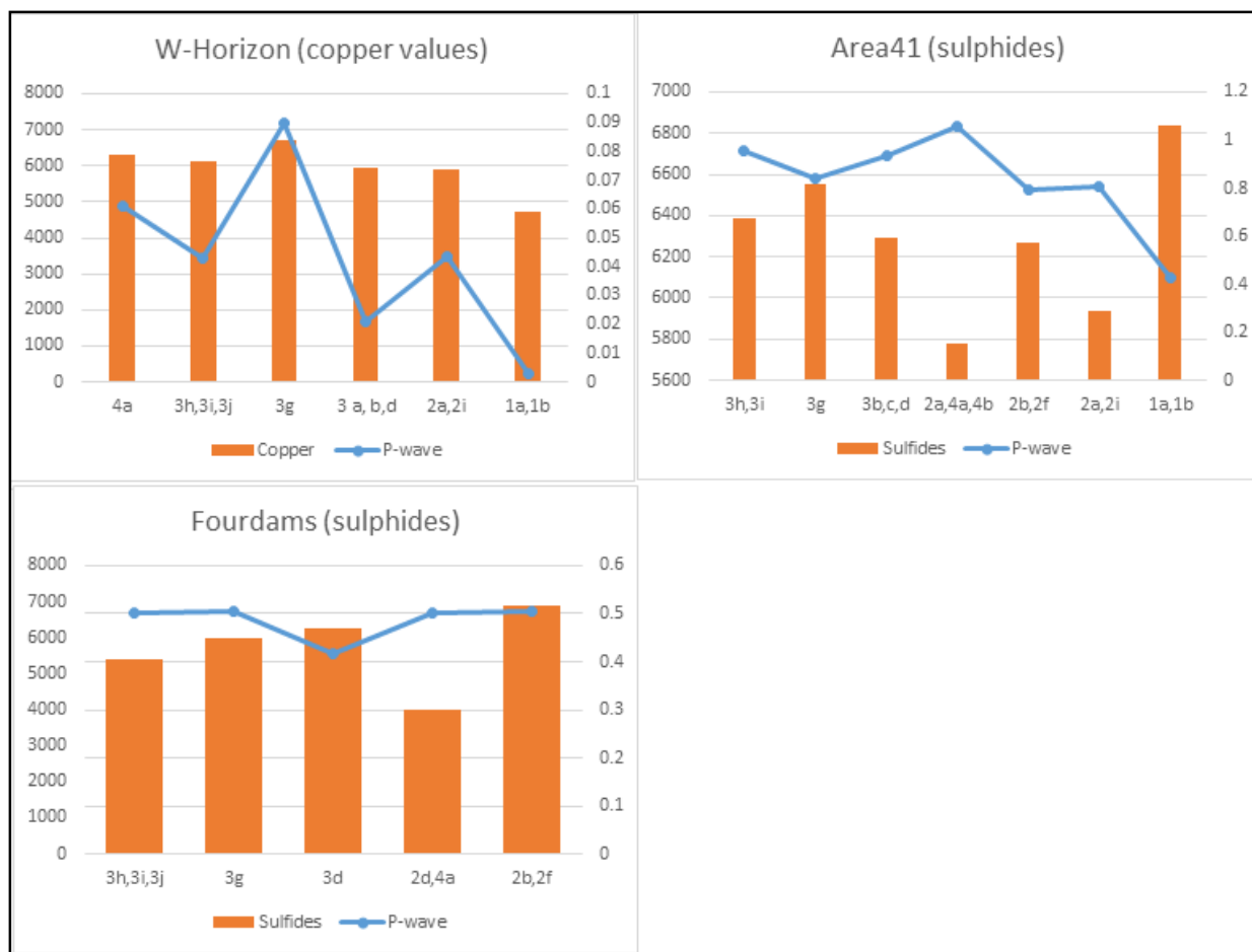
Figure 6.19- P-wave velocity distribution with regards to the sulphur content which is represented by the Sulphur values obtained by assay data for the drill cores
