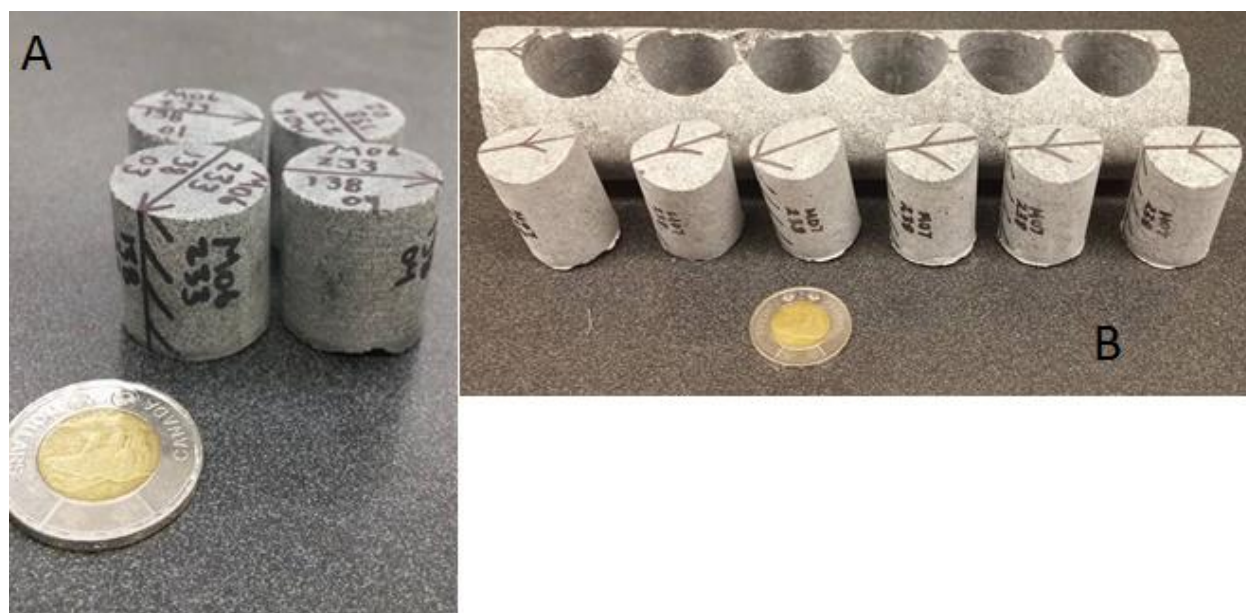
Figure 3.1- A) 10 cm 3 specimens which have been obtained by drilling perpendicular to the drill core axis as is seen in B). The up direction of the drill core is marked on all samples as well as the depth from which the samples were obtained.
