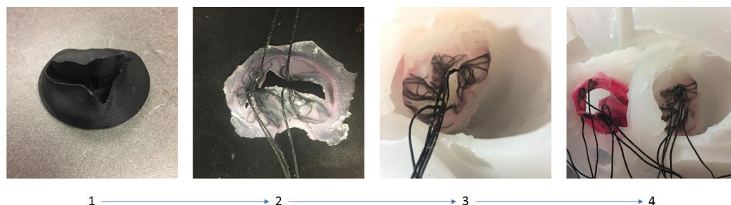
Figure 3.2: Workflow showing the manufacturing of a patient-specific valve model. Step 1 is the 3D printed valve model that is used as a mold. Step 2 is the cured silicone mitral valve model. Step 3 is the mitral valve attached to the full silicone cardiac model. Step 4 shows the silicone mitral and tricuspid valve models inside the silicone heart model.
