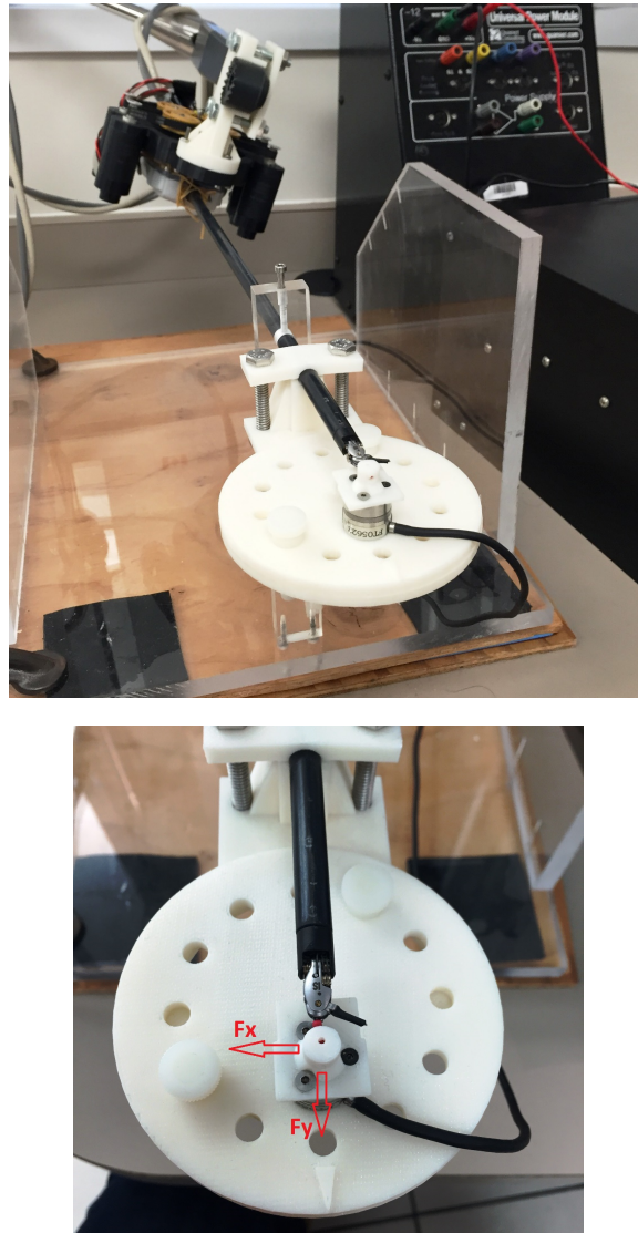
Figure 4.6: The experimental setup: the overall view (top); close-up of the instrument tip fixed to a force sensor (bottom).
