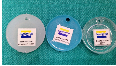
Figure 3.7: The silicone samples used in the first experiment.
