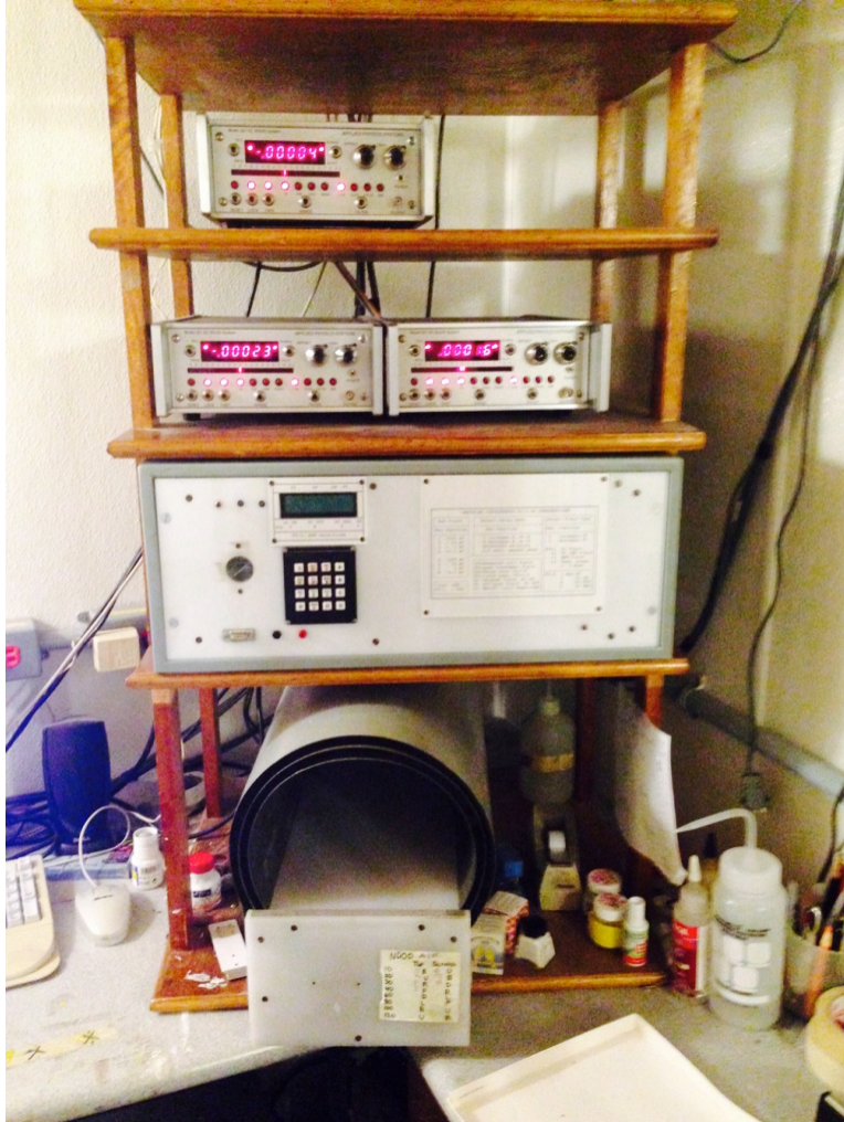
Fig.2.4. Sapphire Instruments SI-4 alternating field demagnetizer at the University of Windsor (bottom two shelves) with cryogenic SQUID controllers for X,Y,Z axes on upper shelves.
