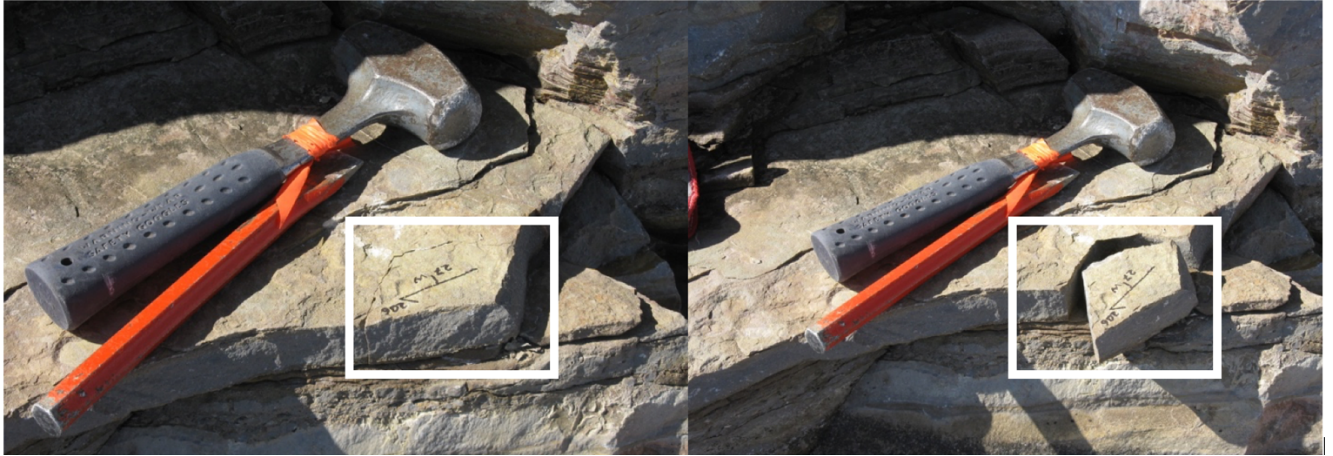
Fig.2.1. Oriented block sampling in which strike and dip measurements are taken prior to removal from outcrop.
