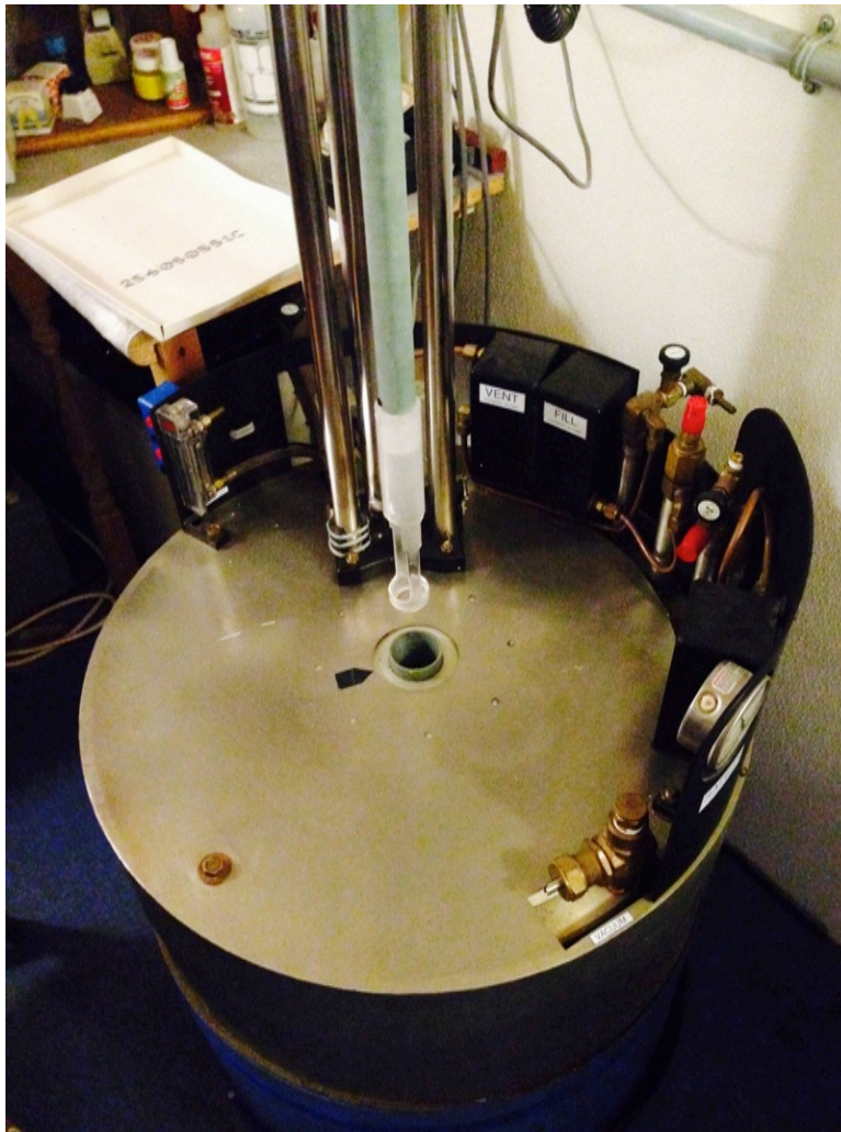
Fig.2.3. 2G Cryogenic magnetometer in the paleomagnetic laboratory at the University of Windsor.
