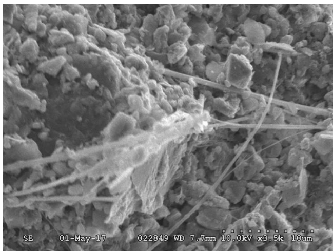
Appendix B-1. SEM photo of 10%-PC-MFT at 28 days, 3500x
