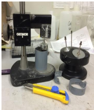
Appendix C-16. Vane shear (Left); Falling cone (Middle); Falling cones (Right)
