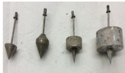
Appendix C-16. Vane shear (Left); Falling cone (Middle); Falling cones (Right)
