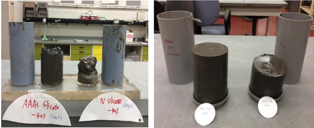
Appendix C-7. 40%-AAAS-MFT and 40%-NS-MFT at 7 days (left); 50%-AAAS-MFT and 60%-AAAS-MFT at 14 days (right)
