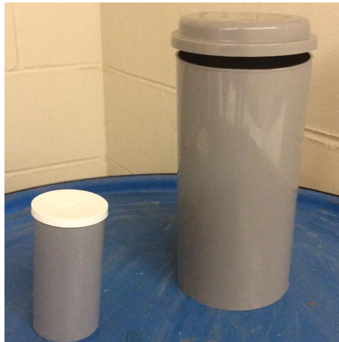
Fig. 4.2 Cylindrical plastic mold for curing, left: 50mm*100mm; Right: 100mm*200mm
