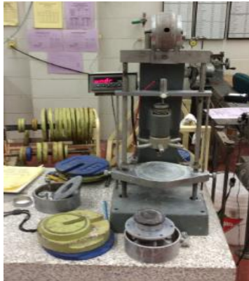
Appendix C-15. Pycnometer (Left); Oedometer (Middle); Supernatant (Right)
