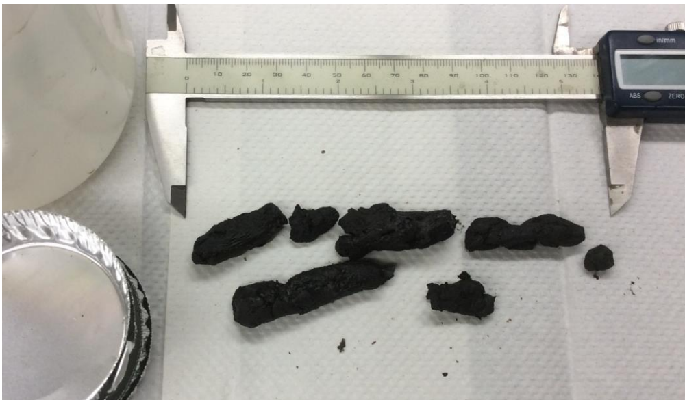
Fig. 5.15 Plastic limit test of MFT samples treated by high amount of silicates
