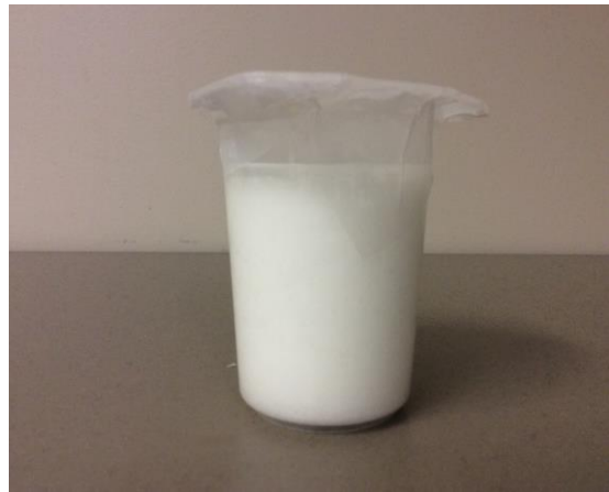
(b): AAAS gel after 60 days curing
