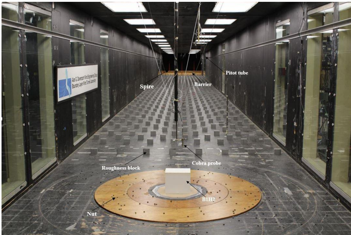
Figure 17: Photograph of the experimental setup of a model in wind tunnel.
