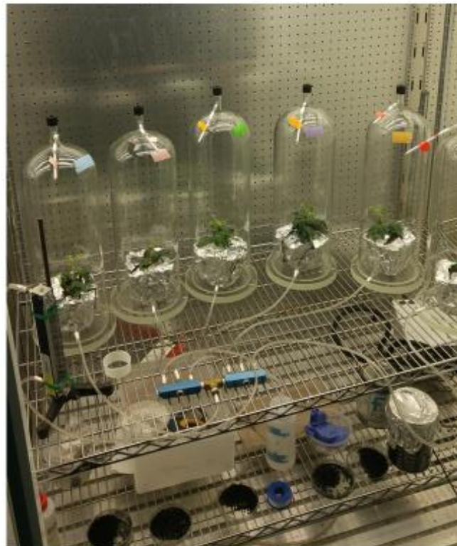
Figure 3. Dynamic Headspace collection chambers containing two plants of each Micro-Tom tomato genotype – WT, CCD1a L1, and CCD1a L2.
