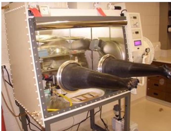
**Figure 2.11** A picture of the glovebox used for battery assembly
