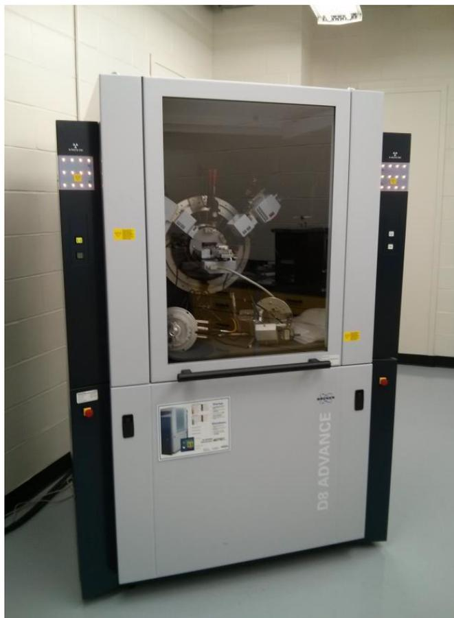
**Figure 2.6 A Bruker D8 Advance Diffractometer XRD**
