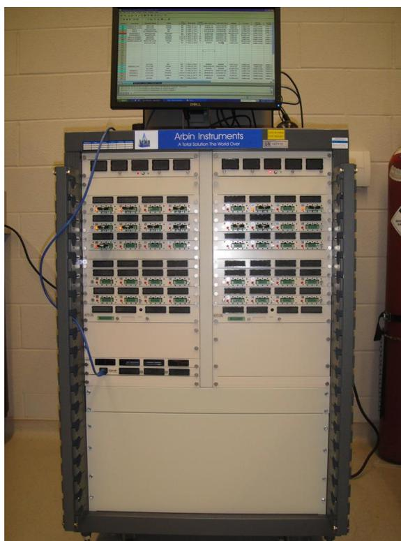
**Figure 2.12 An Arbin BT2000 battery test station**
