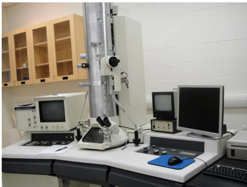
**Figure 2.4 Instrument of a Hitachi H-7000 transmission electron microscope**
