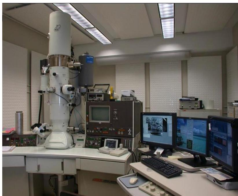
**Figure 2.5 A picture of JEOL 2010F high-resolution TEM**
