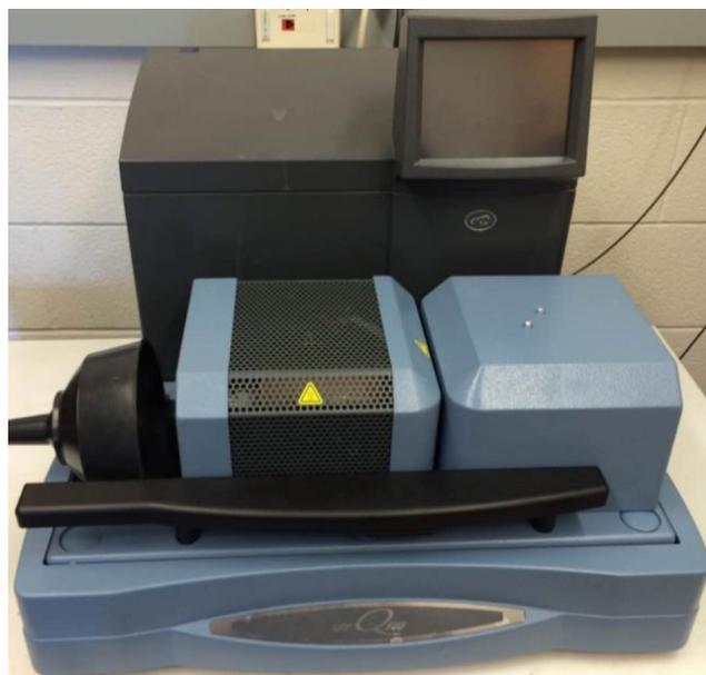
**Figure 2.7 A SDT Q600 Thermogravimetric/Differential Scanning Calorimetry Analyzer**
