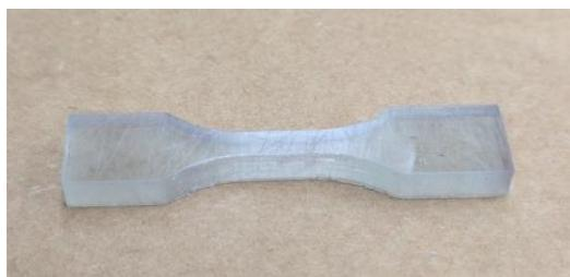
**Fig. 3-6. Test specimen for axial tension experiment.**
