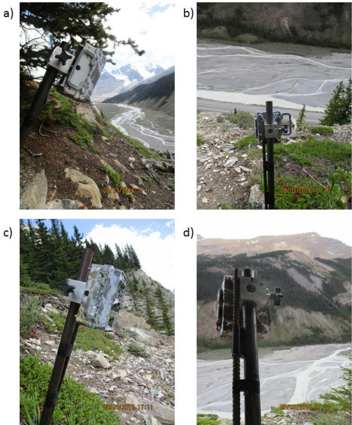
Figure 3.3: Set up of the time-lapse cameras with one viewing upstream (a, b) and the other downstream (c, d) with an area of overlap between the two.
