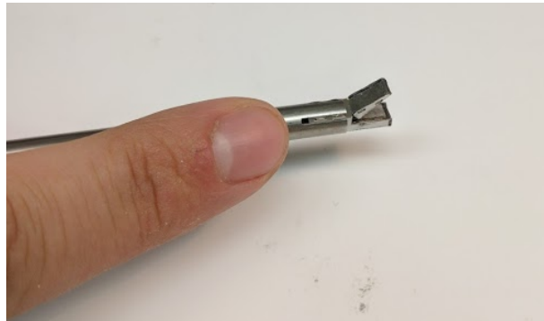
(a): PCMEMS grasper mounted in stainless steel shaft for testing.
