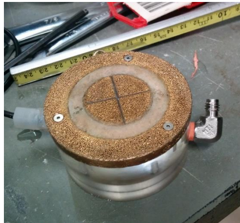
Figure 4.1 PRA device for measuring shear wave velocity
