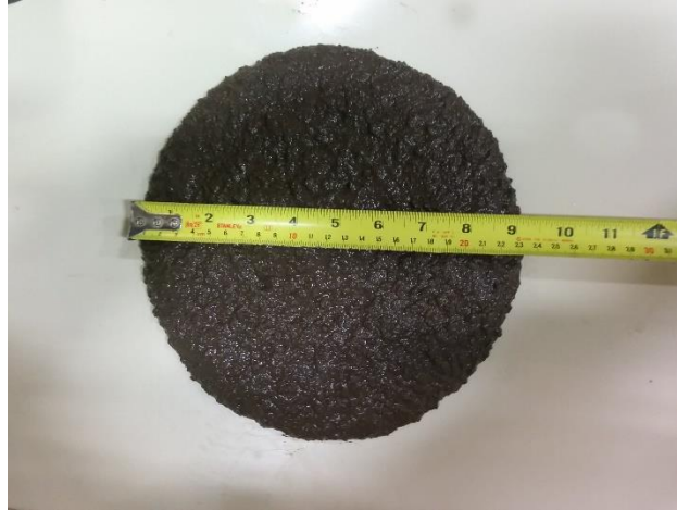
Figure 3.3 Measurement of flowability value of a fresh CLSM mixture
