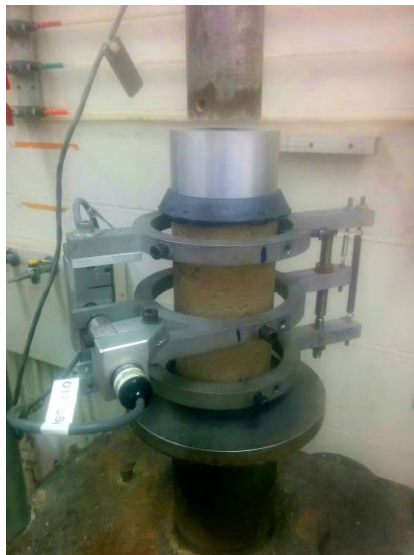
Figure 4.4 Determining static Poisson's ratio using a compressometer
