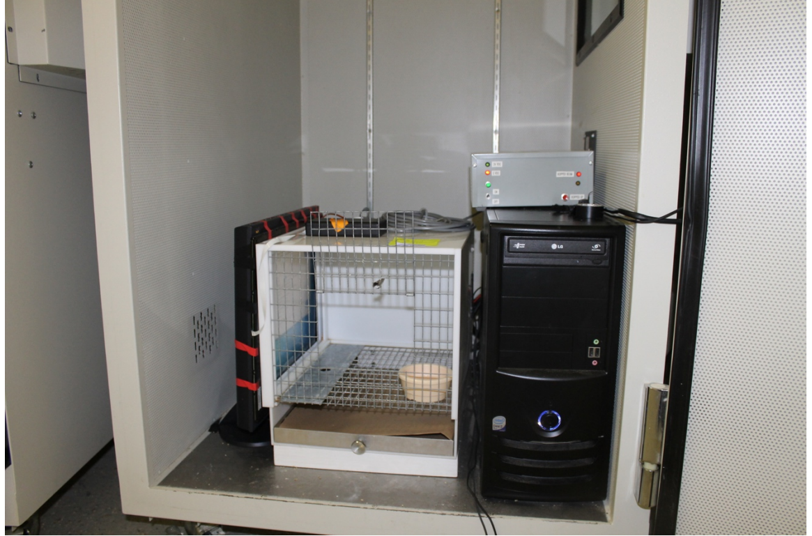
Figure 2.6. Operant chamber, operant control box, touchscreen, touchscreen control hub, inside computer monitor, and computer tower.
