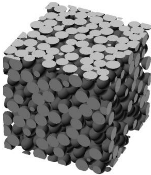
Figure 1.6: CAD model of periodic cubic REV developed by Chueh et al. [37]
