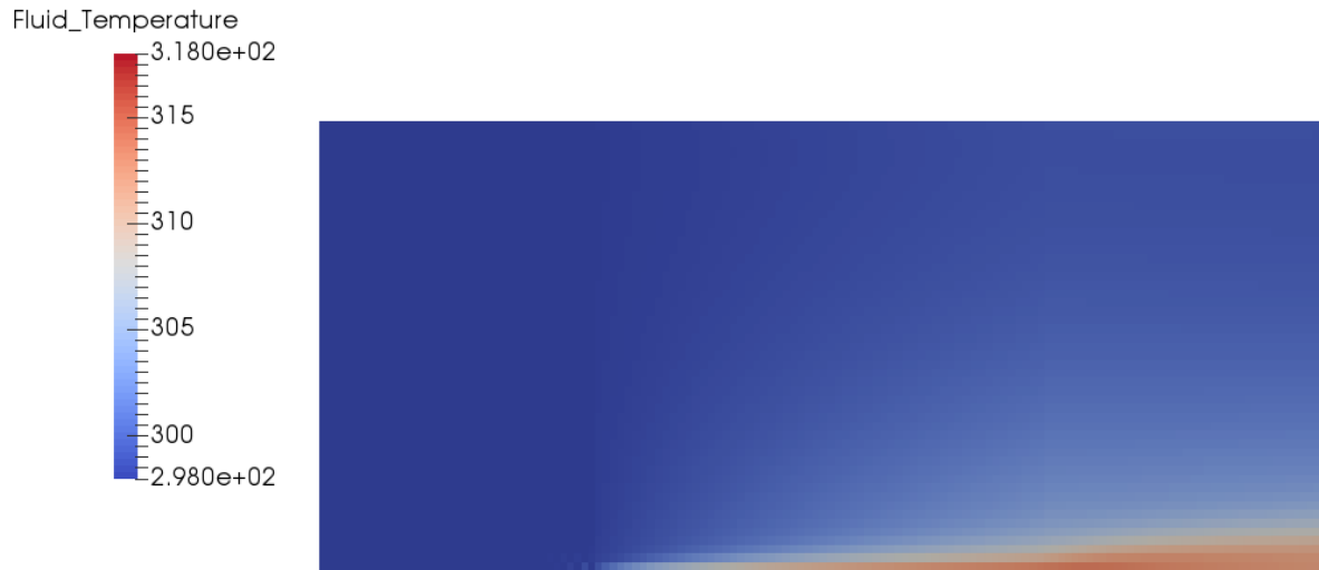
Figure 4.7: Temperature contours obtained from porous continuum model at Re 80, Porosity 0.75, 400-micron diameter, and using water.
