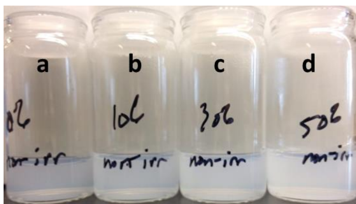
Figure A-12. Celecoxib-containing NPs based on PLA-PEtG-disulfide blends after 4 h. (a) 100% PEtG, (b) 10% PLA-PEtG, (c) 30% PLA-PEtG, and (d) 50% PLA-PEtG.
