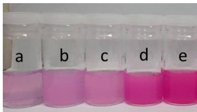
Figure 24. Nile red-loaded PLA-PEtG NP suspensions: (a) 100% PEtG, (b) 10 wt% PLA, (c) 30 wt% PLA, (d) 50 wt% PLA, and (e) 100% PLA.
