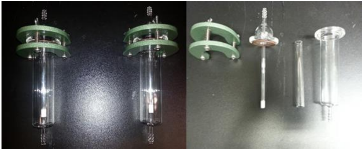
Figure 3.6 Schematic diagram (top) and the photographs (bottom) of the first glass-made adsorption column
