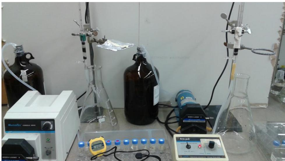
**Figure 1.4: Continuous column adsorption setup**
