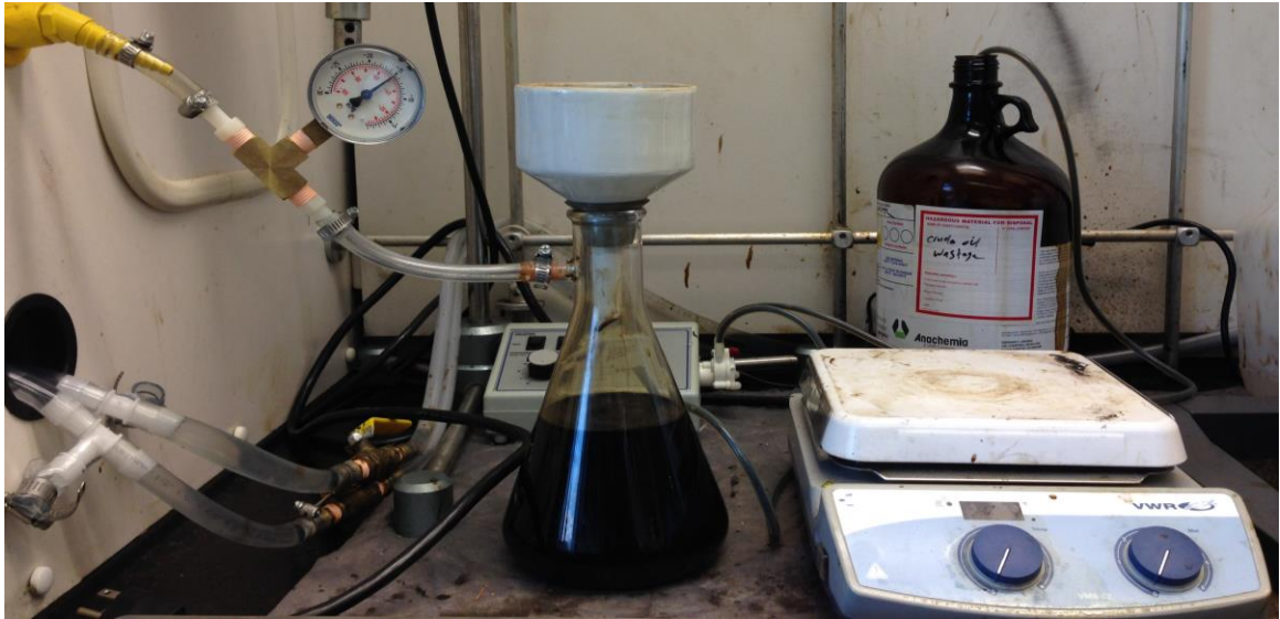
Figure 5-2 Schematic diagram of the experimental setup for asphaltene extraction.
