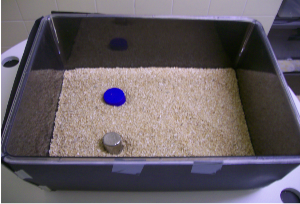
Figure 6: A photograph of the Novel Object Recognition test used to assess recognition memory in mice: The NOR test measures the amount of time spent by a mouse exploring the novel object. In a previous configuration of the above setup, two blue caps are the 'old objects' that the mouse spends time exploring during the first day of testing ('acclimatization'). On the second day of testing (above configuration), a 'novel object,' in this case a shiny bottle cap, replaces one blue cap and the NOR test measures how long the mouse spends exploring the shiny cap. A functioning, healthy recognition-memory performance is indicated by the longer time spent by the mouse exploring the novel object.
