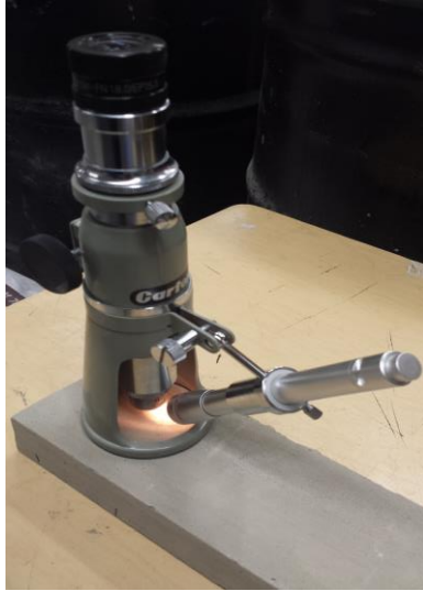
Figure 3-2: Crack monitoring optical microscope.
