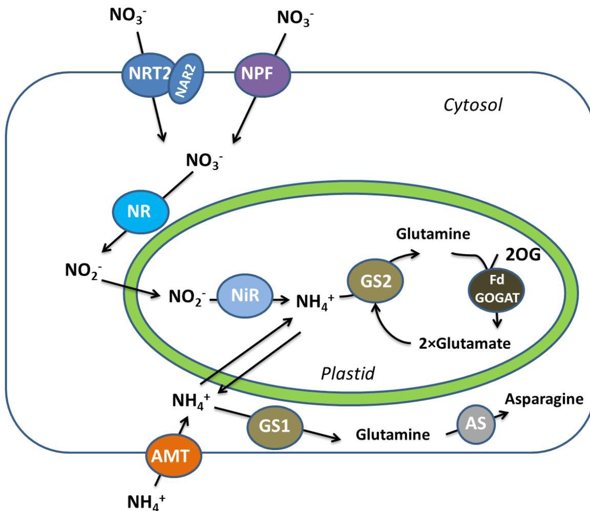
**Figure 1.1** Schematic presentation of enzymes involved in the primary nitrogen assimilation pathway.
