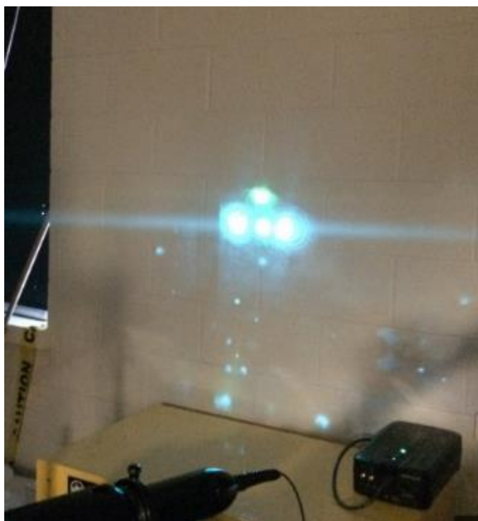
Fig. 2A-8 Projection of the four laser beams against a white flat background to evaluate measurement volume overlap.
