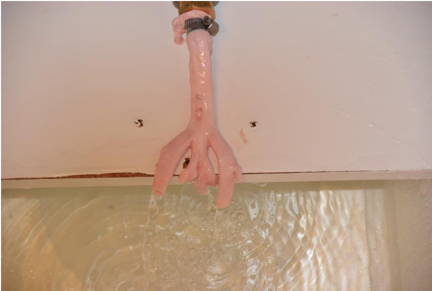
Figure 4.18 Porcine aorta with 1 cm diameter iliac defect with device deployed
