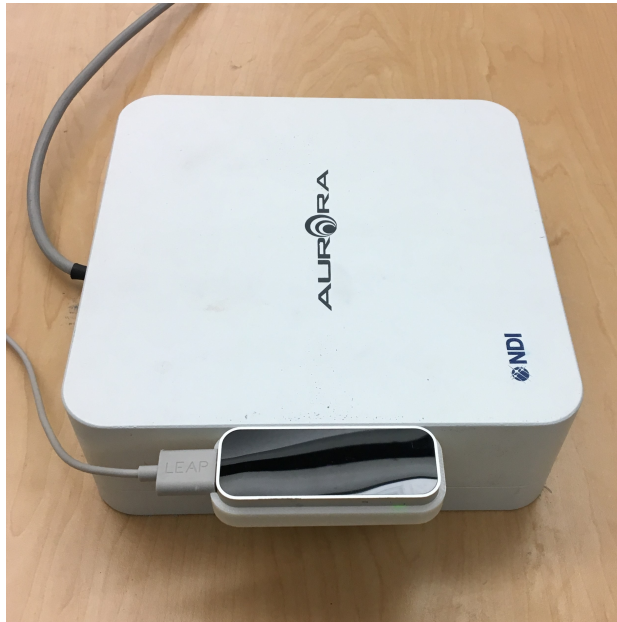
Figure 3.12: Leap Motion controller mounted to Aurora electromagnetic field generator
