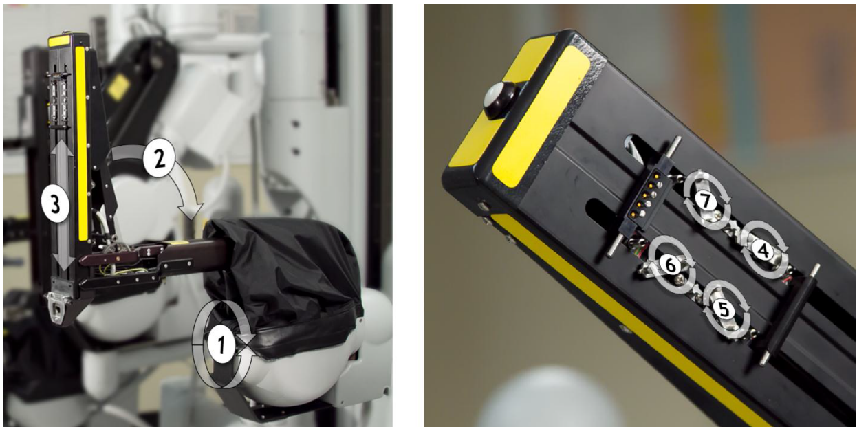
Figure 2.13: Joints of the PSM and their direction of motion (©Intuitive Surgical, Inc.)
