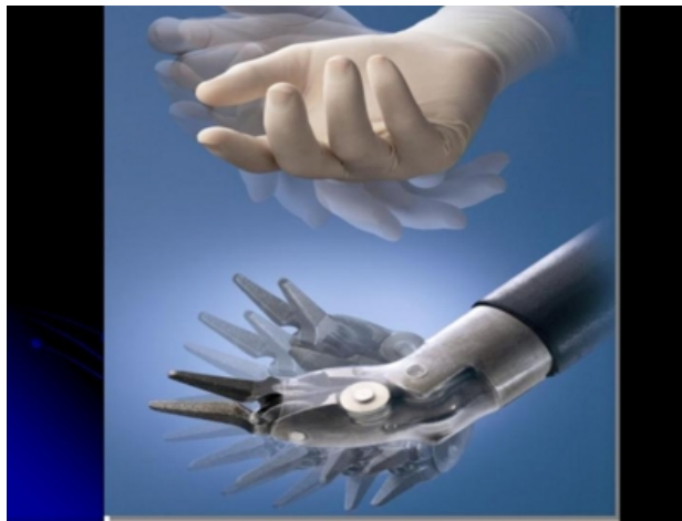
Figure 1.6: Comparing Endowrist ® to the human wrist (©Intuitive Surgical, Inc.)
