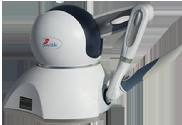
Figure 2.7: Phantom Omni ® haptic device (©Geomagic, Inc.)
