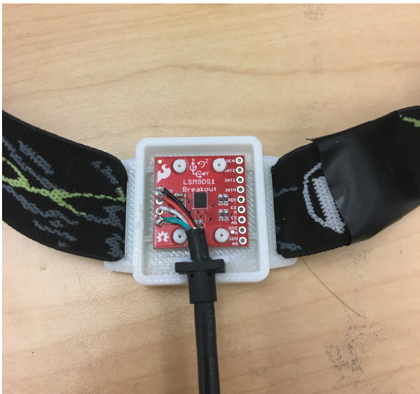
(a) IMU board in 3D printed case
