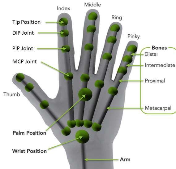
Figure 2.17: Leap motion tracked points (©Leap Motion, Inc.)
