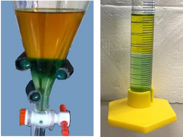
Figure S-14 Photo of lutein extraction and saponification by ether and ethanol after water addition. Left: concentrated solution, Right: 1% (v/v) sample analysis
