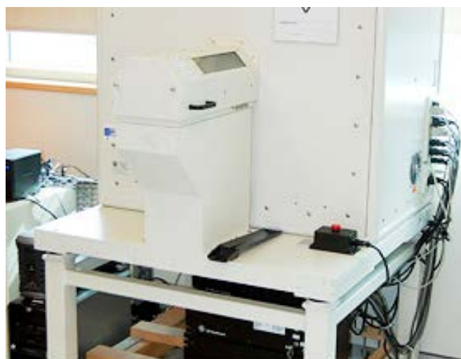
Figure 2.2: GE eXplore Locus \mu CT scanner used for meteorite scans at the Robarts pre-clinical imaging center (Healthcare GE, 2005).
