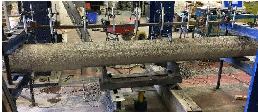
**Figure 5.4 Bending test setup on extracted pile**
