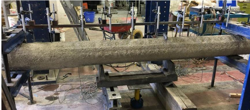
**Figure 5.4 Bending test setup on extracted pile**
