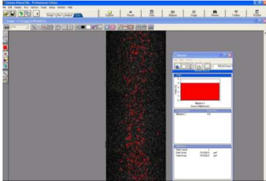
Figure 4.4: The measurement of area fraction on ESGs in the cross section of casting using image analysis software Clemex.
