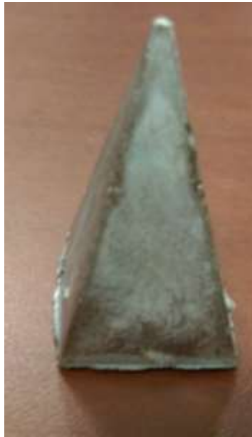
Figure 6.5: Wedge casting under applied pressure 175 bar.
