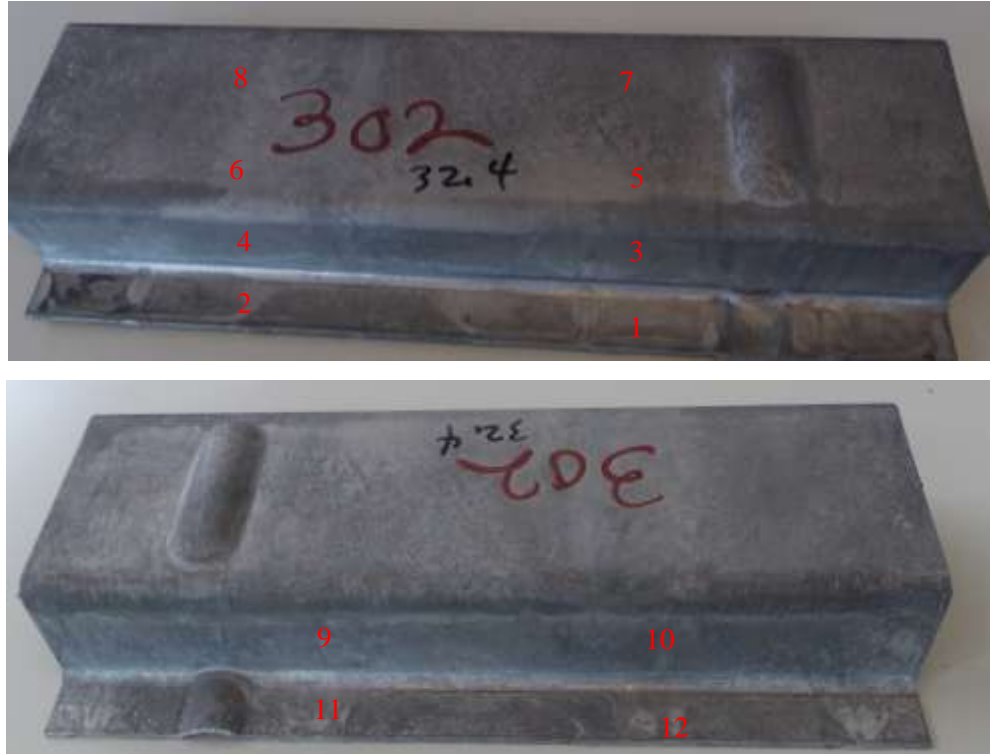
Figure 4.5: Locations of 12 tensile specimens were cut from a die-cast Top hat from gate to overflow.
