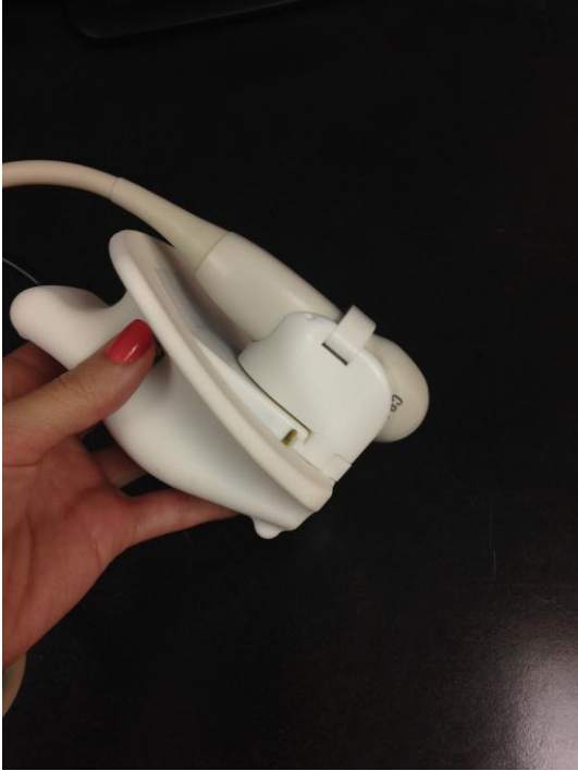
Figure 6-1 - Clinical 2D US transducer within the hand-held motorized transducer housing simulating a scan of a preterm sized mannequin.
