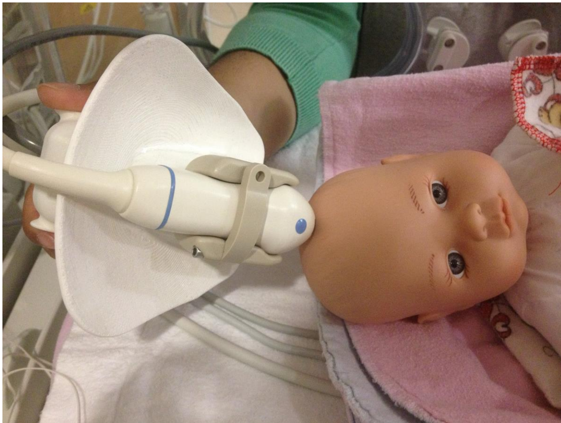
Figure 3-1– Mechanical 3D US transducer housing with transducer in place. This entire housing/transducer set up done through incubator port holes in order to mimic scan with minimal disruption to patient.
