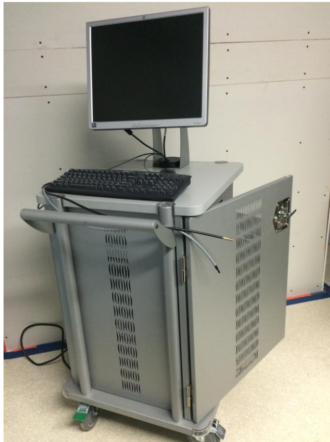
Figure 2.2: In-house developed, continuous-wave broadband NIRS system mounted on a cart for bedside use, consisting of a diffraction grating spectrometer (Sciencetech Inc., ON, Canada), coupled to a charge coupled device (CCD) camera (Wright Instruments, UK).
