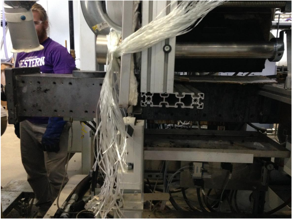
Figure 3-5 The second extruder (ZSG) of Dieffenbacher D-LFT-ILC line.
