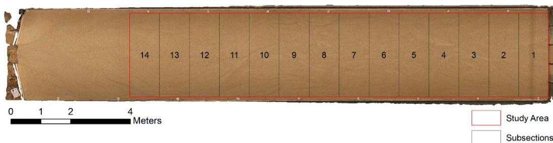
**Figure 5.11 – The flume study area divided into 14 x 1 m slices for sediment budgeting.**
