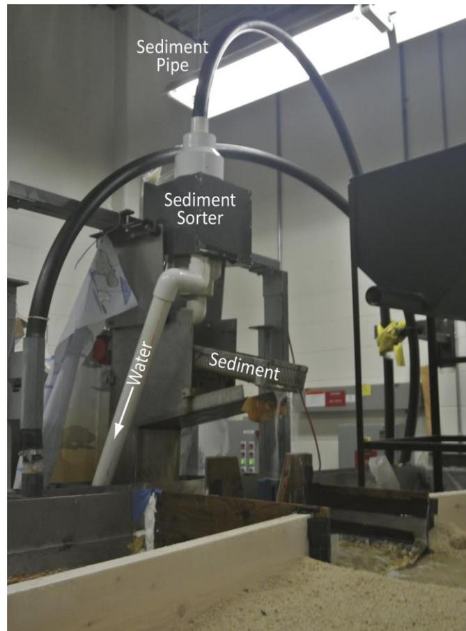
**Figure 3.7 – Image of the upstream sediment sorter. A water and sediment mixture from the sediment pump is propelled through the sediment pipe into the sorter. The sorter returned water to the head tank as sediment rolled down a slide onto the weir.**
