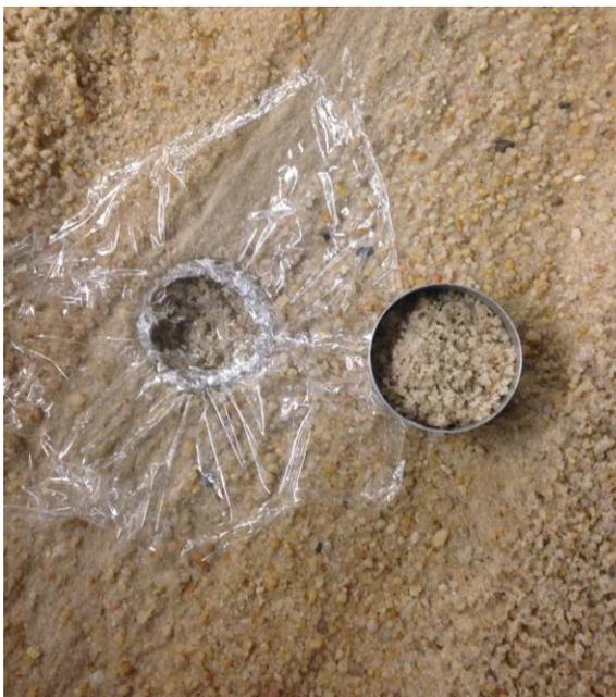
**Figure H.1 – Water replacement method for the estimating bulk density. Sediment removed from the hole was collected and the hole was lined with plastic and filled with water.**
