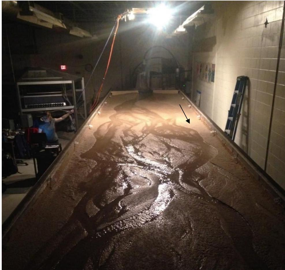
**Figure 3.17 – Demonstration of a wet photo survey being completed at the end of an experimental run. Arrow indicates flow direction.**
