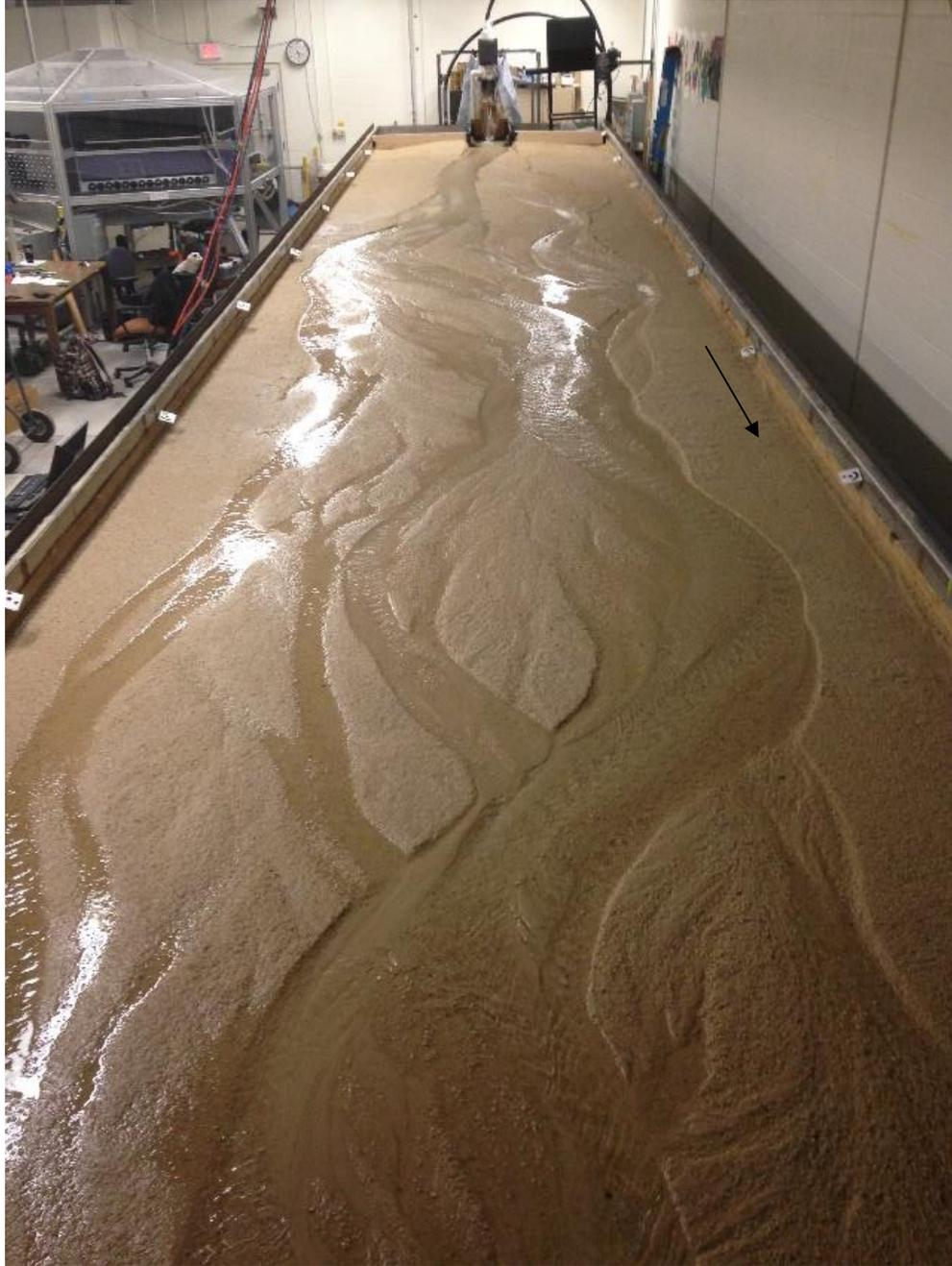
**Figure 3.1 – Image of the physical gravel-bed river flume in the Boundary Layer Wind Tunnel Laboratory at the University of Western Ontario. Arrow indicates flow direction.**
