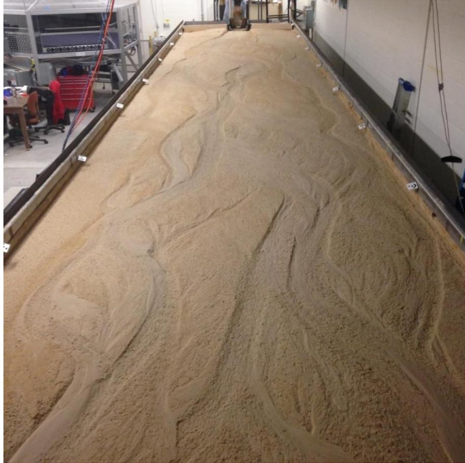
**Figure 3.16 – Example of a dry flume surface from experiment 11. Image taken from the downstream end facing upstream.**
