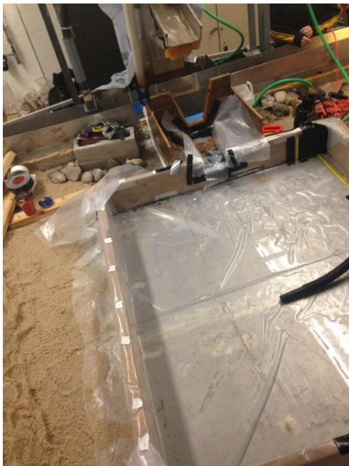
**Figure B.1 – Weir calibration using a custom-built pool.**
