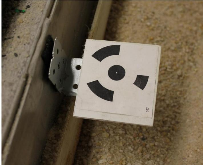
**Figure 3.12 – Example of a coded target in the flume used for digital photogrammetry georeferencing.**
