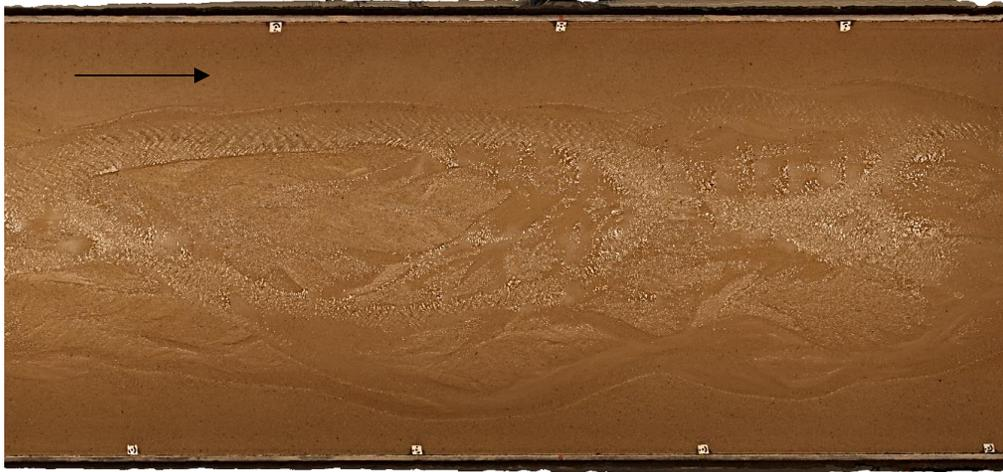
**Figure 3.27 – Example of a wet bed orthophoto created from a wet bed photo survey. This orthophoto was taken from experiment 11 and the arrow indicates flow direction.**
