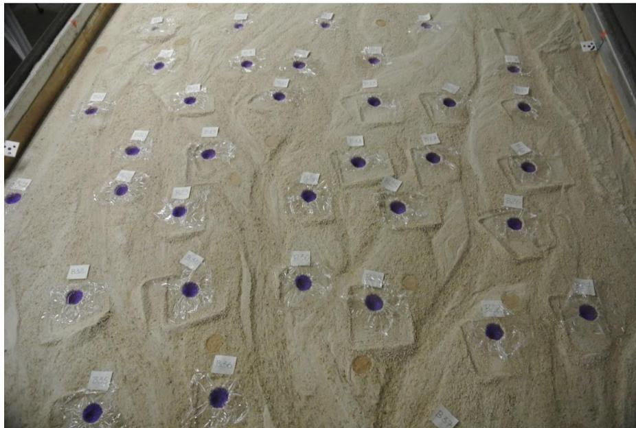
**Figure H.3 – Bulk density sample locations. The bulk density samples were taken at the end of experiment 13, covering a range of morphological features including bars and in-channel locations. The water was dyed purple to improve the visibility of the water against the sand.**
