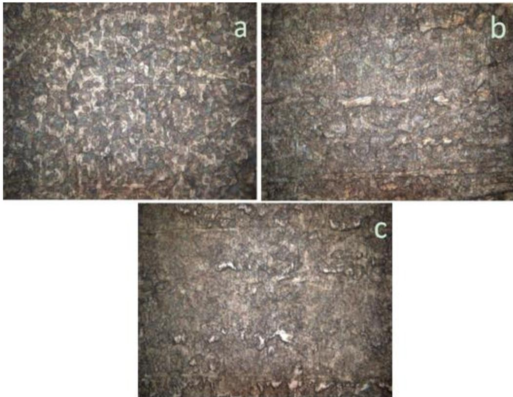
**Figure 6.10** Microscope images of sample I with 500 magnifications under cycles' abrasion: a. before abrasion; b. 300 cycles; c. 500 cycles. Most of the coating was rubbed out after 500 cycles abrasion.
