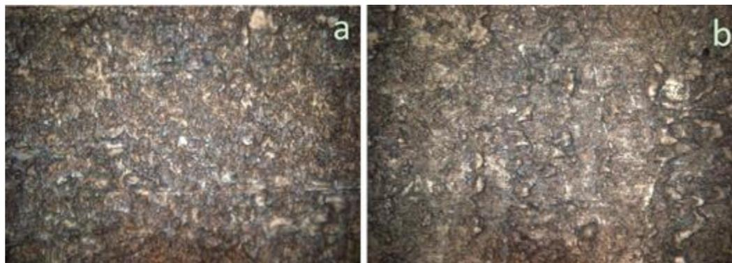
**Figure 6.8** Contrastive images of sample III before and after the 6H pencil scratch with 500 magnifications: a. before the scratch; b. after the scratch. The coated surfaces were harder than 6H since no obviously scratch mark was left on the surface.
