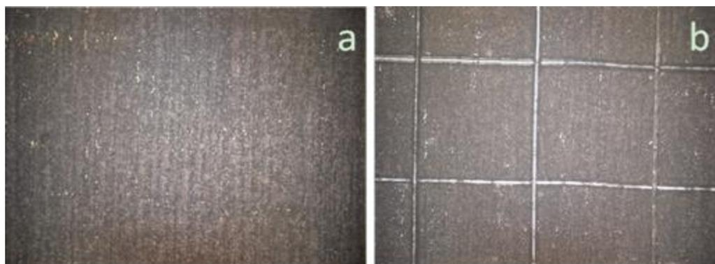
**Figure 6.9** Comparative images of sample III before and after the cross hutch cutter test with 50 magnifications: a. before the test; b. after the test. The silica-titania surface was tightly attached to the titanium substrate.
