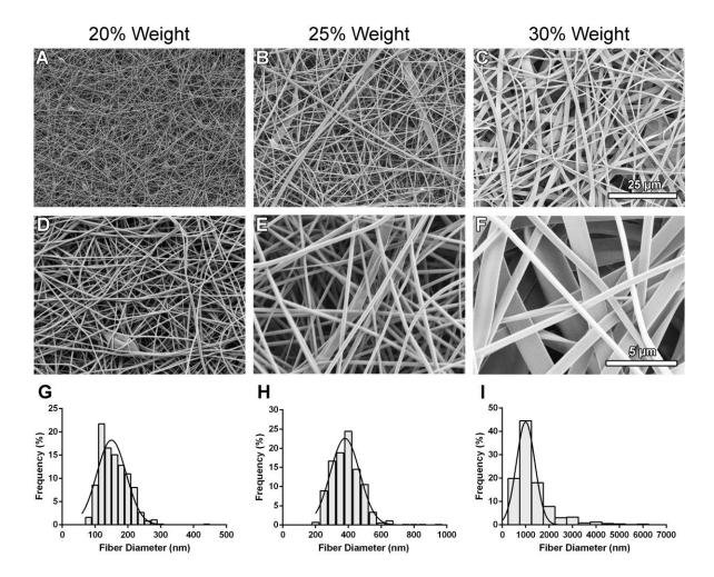
**Figure 2.5** – **Refined scaffold morphology and fiber size distribution:** (A) SEM image of a scaffold electrospun using a flowrate of 0.5 mL/h, a collector distance of 10 cm, and a gelatin concentration of 21% weight. Scale Bar: 15 μm. (B) Frequency distribution graph showing the percentage of fiber diameters within each bin range for scaffolds electrospun using a flowrate of 0.5 mL/h, a collector distance of 10 cm, and a gelatin concentration of 21% weight. N=3, n=250. Bin size: 20 nm.
