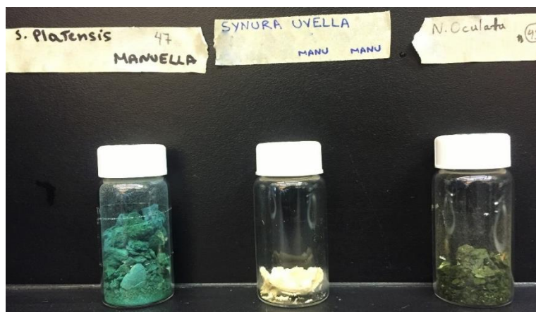
Figure 2.5: Freeze dried biomass of blue-green Spirulina platensis , yellow Synura uvella , green Nannochloropsis oculata .
