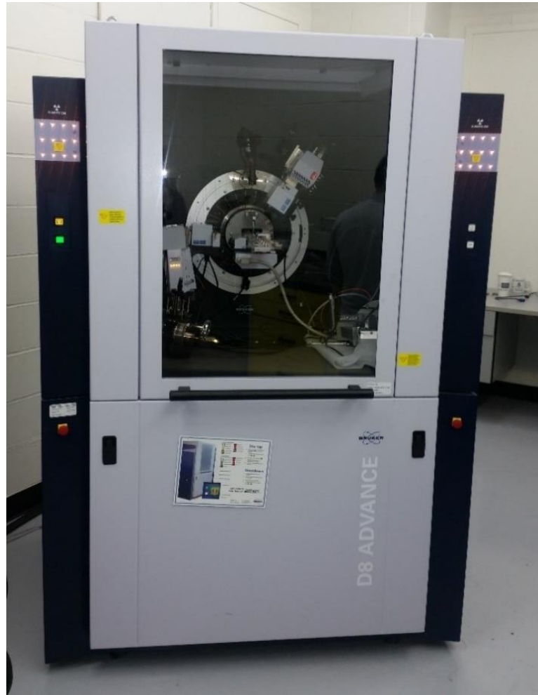
Figure 3.8: Bruker XRD D8 Advance used for composition studies of the coating.
