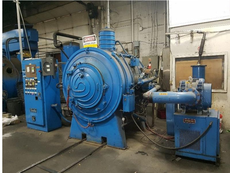
Figure 3.2: Vacuum furnace employed for aging treatment.
