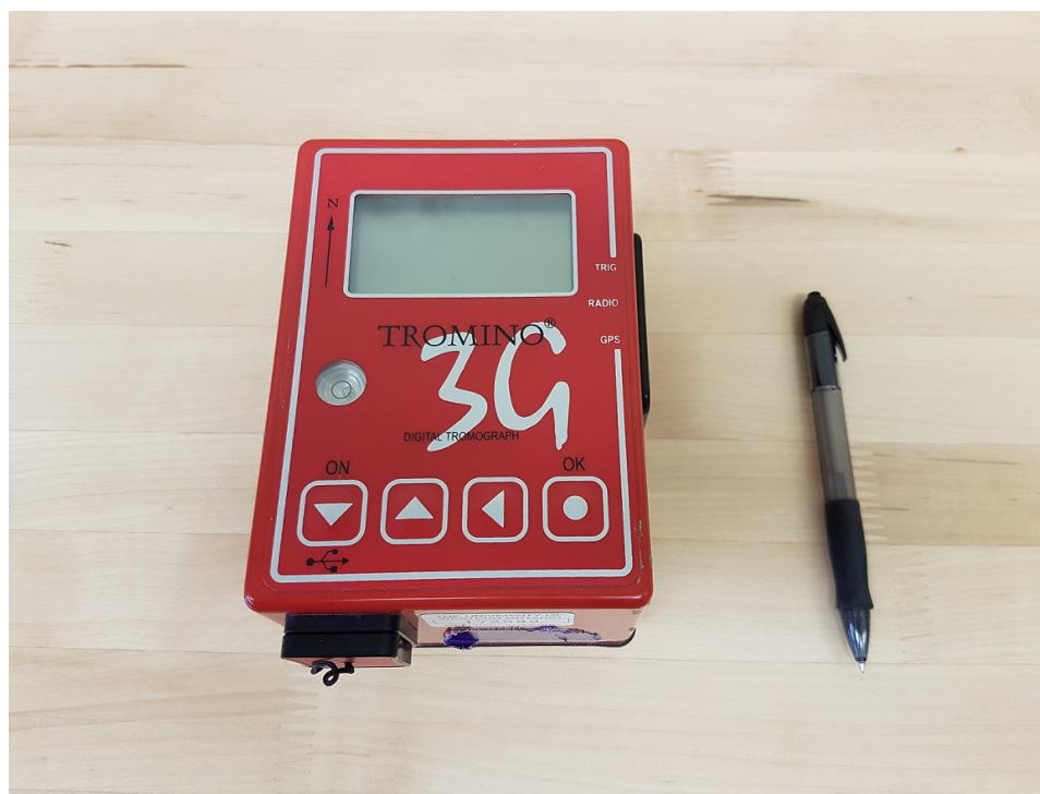
Figure 4-3: The MoHo s.r.l. Tromino ® used to perform ambient noise surveys in this study.
