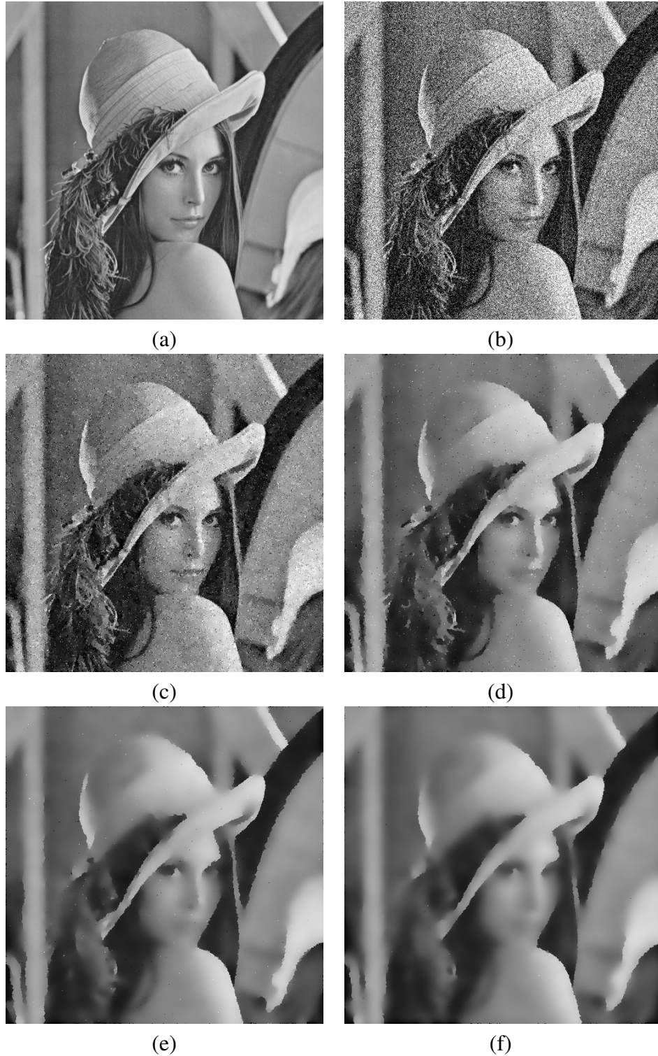
Figure 2.10: The effects of K on ADF: (a) an original Lena image, (b) an AWGN noisy image with \sigma = 20 , (c) a denoised image using ADF ( iterations = 100, \lambda = 0.25 , k = \mathbf{0.02} ), (d) a denoised image using ADF ( iterations = 100, \lambda = 0.25 , k = \mathbf{0.03} ), (e) a denoised image using ADF ( iterations = 100, \lambda = 0.25 , k = \mathbf{0.04} ), and (f) a denoised image using ADF ( iterations = 100, \lambda = 0.25 , k = \mathbf{0.05} ).
