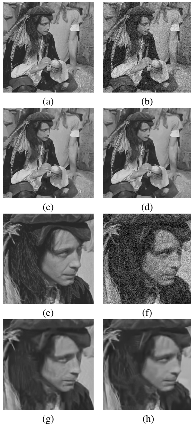
Figure 6.3: The results of denoising the Man image at noise level ( \sigma = 30 ): (a) noise-free Man image 512 \times 512 , (b) AWGN noisy image ( \sigma = 30 ), (c) BM3D, (d) our method, and (e), (f), (g) and (h) fragments images of the first rows
