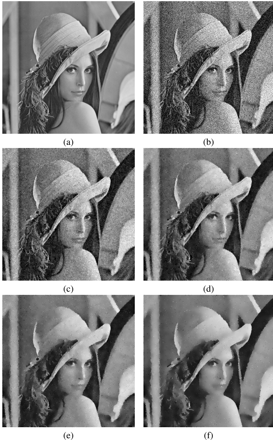
Figure 2.11: The effects of \lambda on ADF: (a) an original Lena image, (b) an AWGN noisy image with \sigma = 20 , (c) a denoised image using ADF ( iterations = 100, \lambda = \mathbf{0.10} , k = 0.03 ), (d) a denoised image using ADF ( iterations = 100, \lambda = \mathbf{0.15} , k = 0.03 ), (e) a denoised image using ADF ( iterations = 100, \lambda = \mathbf{0.20} , k = 0.03 ), and (f) a denoised image using ADF ( iterations = 100, \lambda = \mathbf{0.25} , k = 0.03 ).
