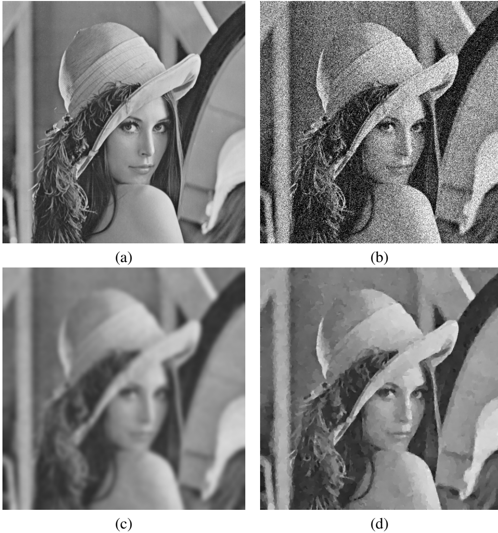
Figure 3.2: Isotropic heat diffusion and TV filtering: (a) an original Lena image, (b) an AWGN noisy image with \sigma = 20 , (c) a denoised image using heat diffusion ( iteration = 50, \Delta t = 0.2 ), and (d) a denoised image using a TV filter ( iteration = auto (121), \lambda = 0.02 , \Delta t = 0.2 ).
