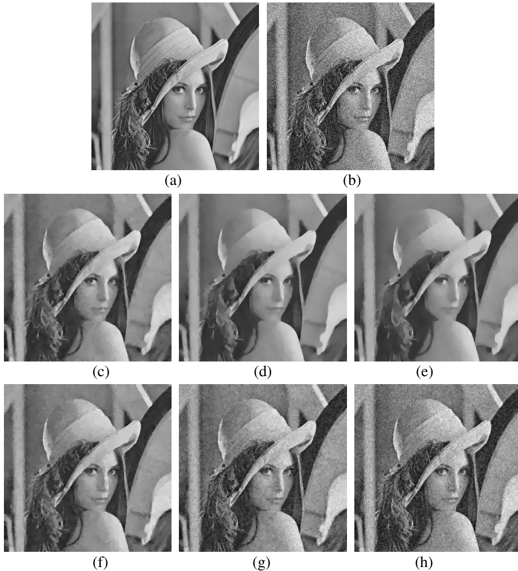
Figure 2.7: TV method for image denoising: (a) an original Lena image, (b) an AWGN noisy image with \sigma = 20 , (c) a denoised image using a TV filter ( iteration = 50, \lambda = auto, \Delta t = 0.2 ), (d) a denoised image using a TV filter ( iteration = auto(127), \lambda = auto, \Delta t = 0.2 ), (e) a denoised image using a TV filter ( iteration = 200, \lambda = auto, \Delta t = 0.2 ), (f) a denoised image using a TV filter ( iteration = auto(121), \lambda = 0.02, \Delta t = 0.2 ), (g) a denoised image using a TV filter ( iteration = auto(122), \lambda = 0.03, \Delta t = 0.2 ), and (h) a denoised image using a TV filter ( iteration = auto(108), \lambda = 0.04, \Delta t = 0.2 ).
