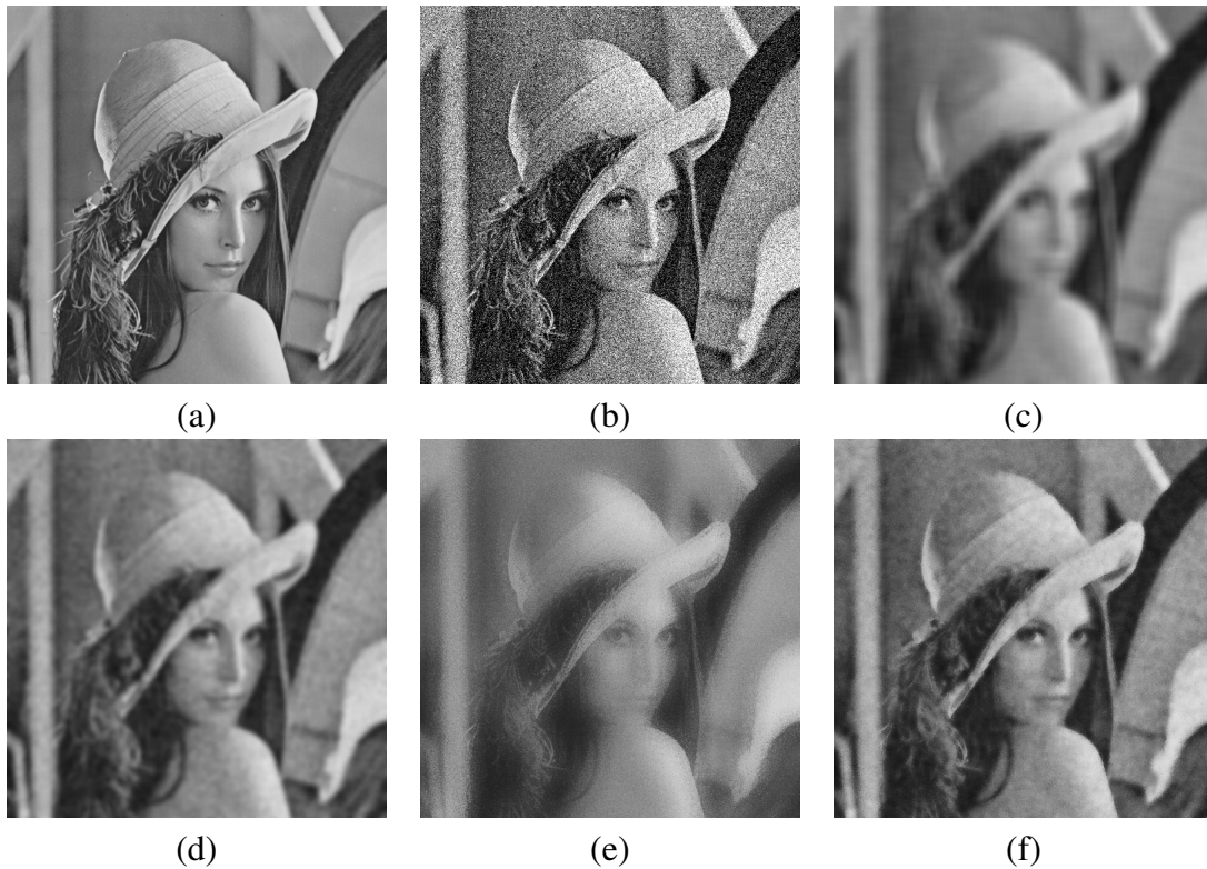
Figure 3.1: Low-pass vs. BF: (a) an original Lena image, (b) an AWGN noisy image with \sigma = 20 , (c) a denoised image using a 21 \times 21 mean filter, (d) a denoised image using a 21 \times 21 Gaussian filter \sigma_d = 3.33 , (e) a denoised image using a 21 \times 21 Yaroslavsky filter \sigma_s = 0.5 , and (f) a denoised image using a 21 \times 21 , \sigma_d = 3.33 and \sigma_r = 0.5 BF. \sigma_d controls the space similarity for the blurring strength, and \sigma_r controls the intensity similarity for the edge preserving.
