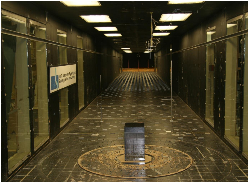
Figure 2-5: Photograph of the wind tunnel with the model inside facing a 180 degree angle. This image shows the exposure used in the background. This terrain configuration involved the barriers, block heights, scattered nuts and spires. The model is set in a 6 panel high configuration ( H/W = 1.66 ).
