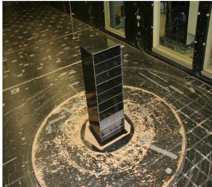
Figure 2-1: Picture of wind tunnel model at tallest H/W configuration with the pressure tap panel 3 rd from the bottom.
