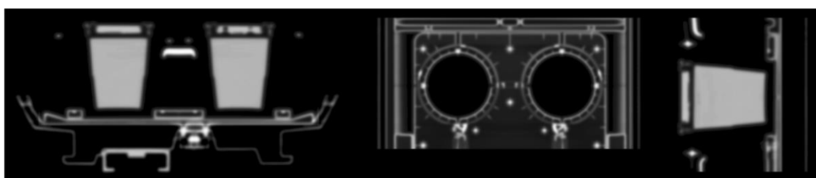
Figure 2-4: Axial, coronal, and sagittal views of a \mu -map composed of manufacturer's table \mu -map, the SECT-based breast coil \mu -map, and the phantom \mu -map fused into a single volume.
