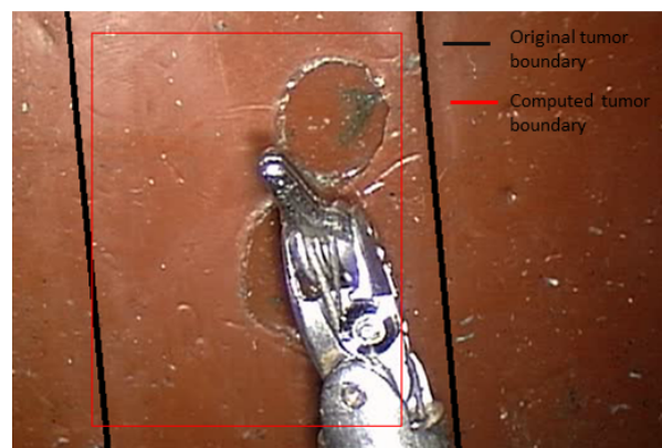
Figure 2.28: The original tumor boundary and the tumor boundary computed using the framework for a palpated section of the phantom.
