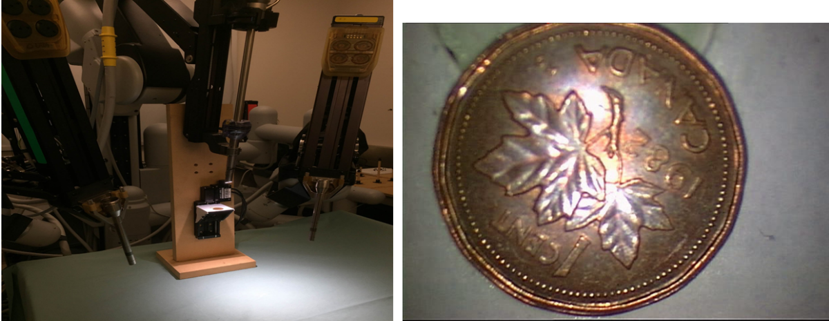
Figure 2.16: Experimental setup for depth validation using linear stage motion.
