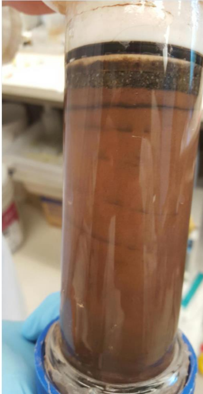
Figure C4: Formation of sulfide precipitate veins in Column B after Experiment 2 (amended).
