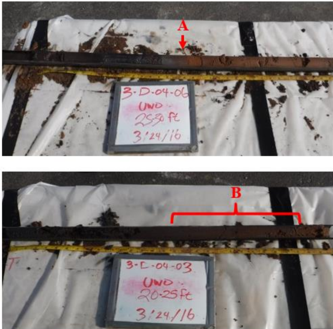
Figure 3.5: Soil cores revealing the contrast between the STAR-treated and untreated soil zones. (Top) Core from IP06 obtained 138 days after STAR, exhibiting a sharp transition between treated and untreated zones (A); (Bottom) core from IP03 also obtained 138 days after STAR exhibits a more gradual transition between the two zones. The total length of core shown is ~1.5m, with depth below ground surface increasing to the right
