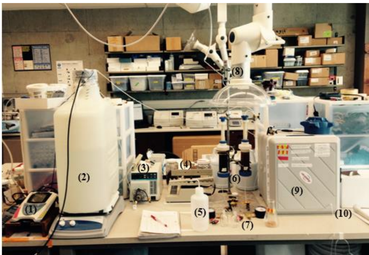
Figure C1: Overview of column setup prior to experimental commencement. Proceeding from left to right, significant items include: (1) probes to measure artificial groundwater (AGW) parameters, (2) AGW reservoir, (3) peristaltic pump used to flow AGW (4) syringe pump, used only for delivering lactate pulses, (5) 70% EtOH used for disinfection of gloves prior to any interactions with the experimental setup, (6) columns A and B, directly following soil packing and prior to being wrapped in tin foil, (7) various valves used to direct flow from the peristaltic and syringe pumps to the appropriate columns, (8) rotameter used to control nitrogen gas flow rate, (9) electric cooler used for collecting samples and sterivex filtering, and (10) effluent line from sterivex filter to collection vessel.
