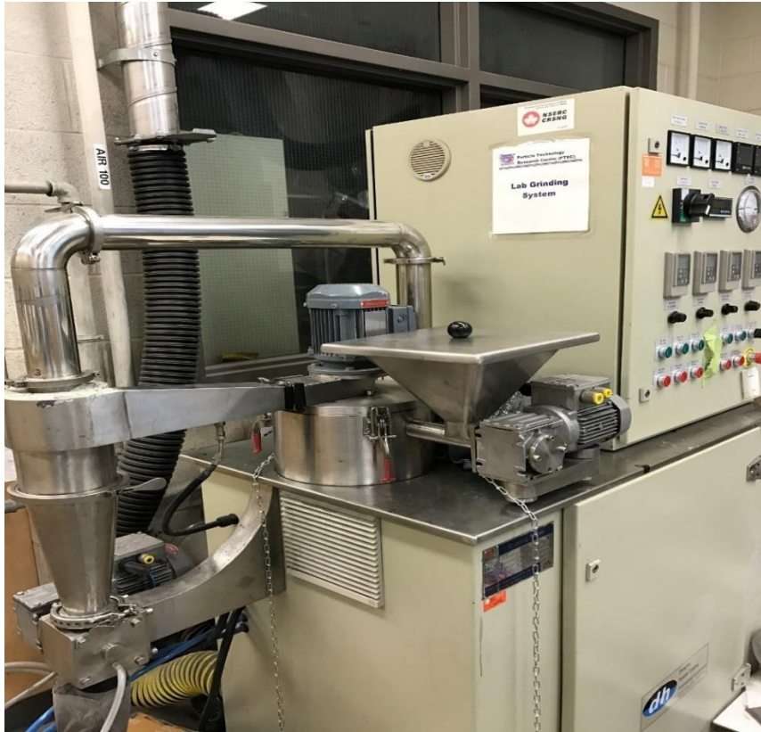
Figure 3.6. Air classifying mill (ACM)
