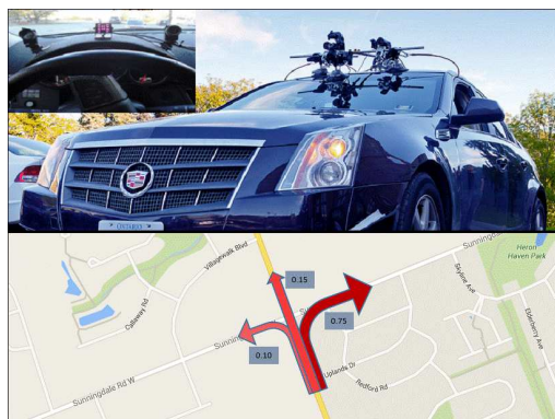
Figure 5.1: (top): Our Vehicular instrumentation configuration. (bottom): Anticipating the probabilities of different driving manoeuvres using vehicle dynamics and driver cephalo-ocular behaviour.
