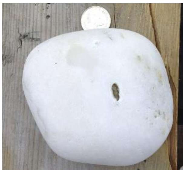
Figure 2-4. A pure quartz prepared to test the contamination during pXRF analysis.
