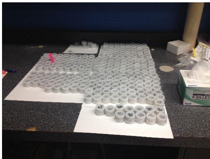
Figure 2-3. Powders in cups that are ready for pXRF analysis.
