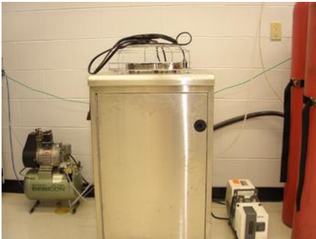
Figure 2.2 Savannah 100 ALD system (Cambridge Nanotech, USA)
