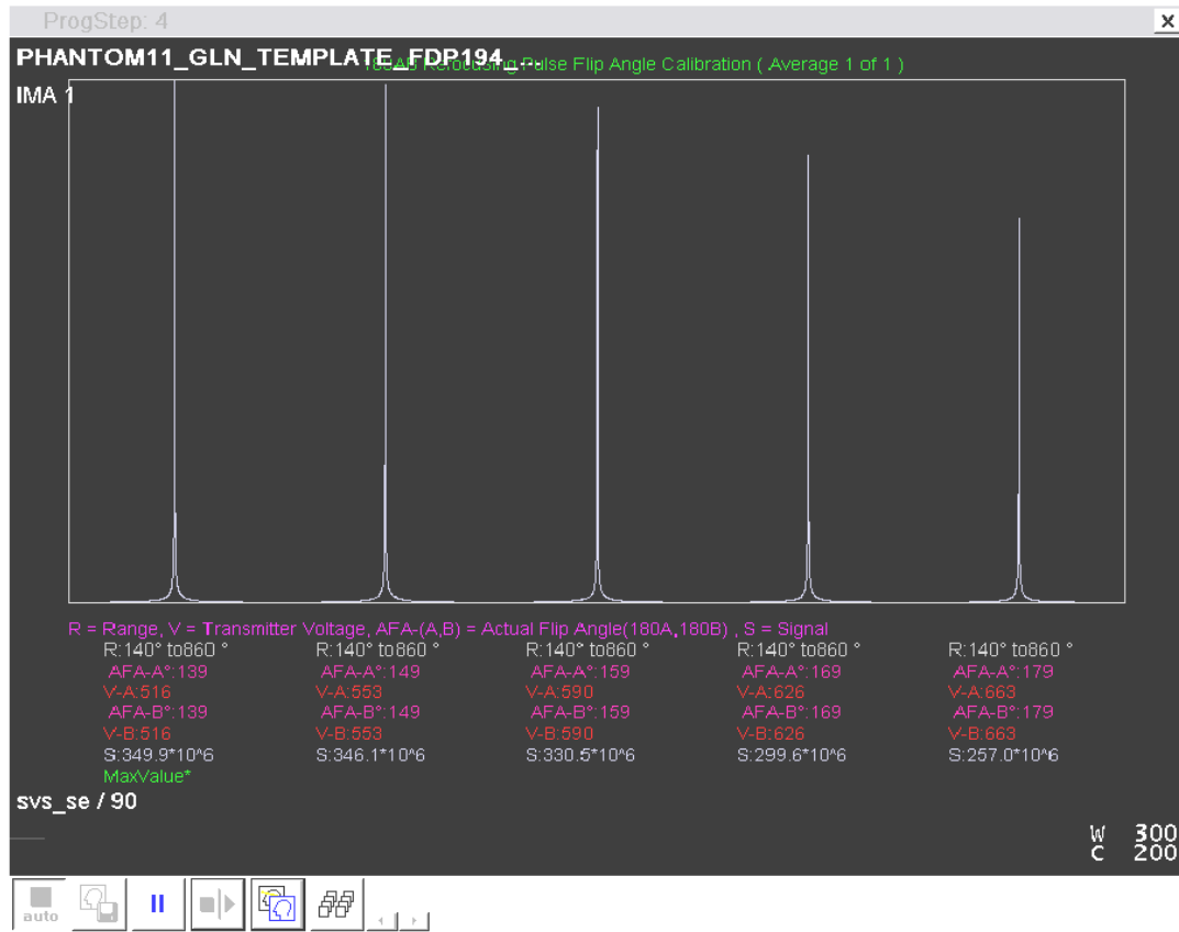
Figure C-4. The inline display illustrates the RF pulse’s flip angle (FA) value, indicating the production of the maximum signal along with the actual FA (AFA), transmitter voltage (V), the signal value (S), and highlights the maximum value with a green label (MaxValue*).
