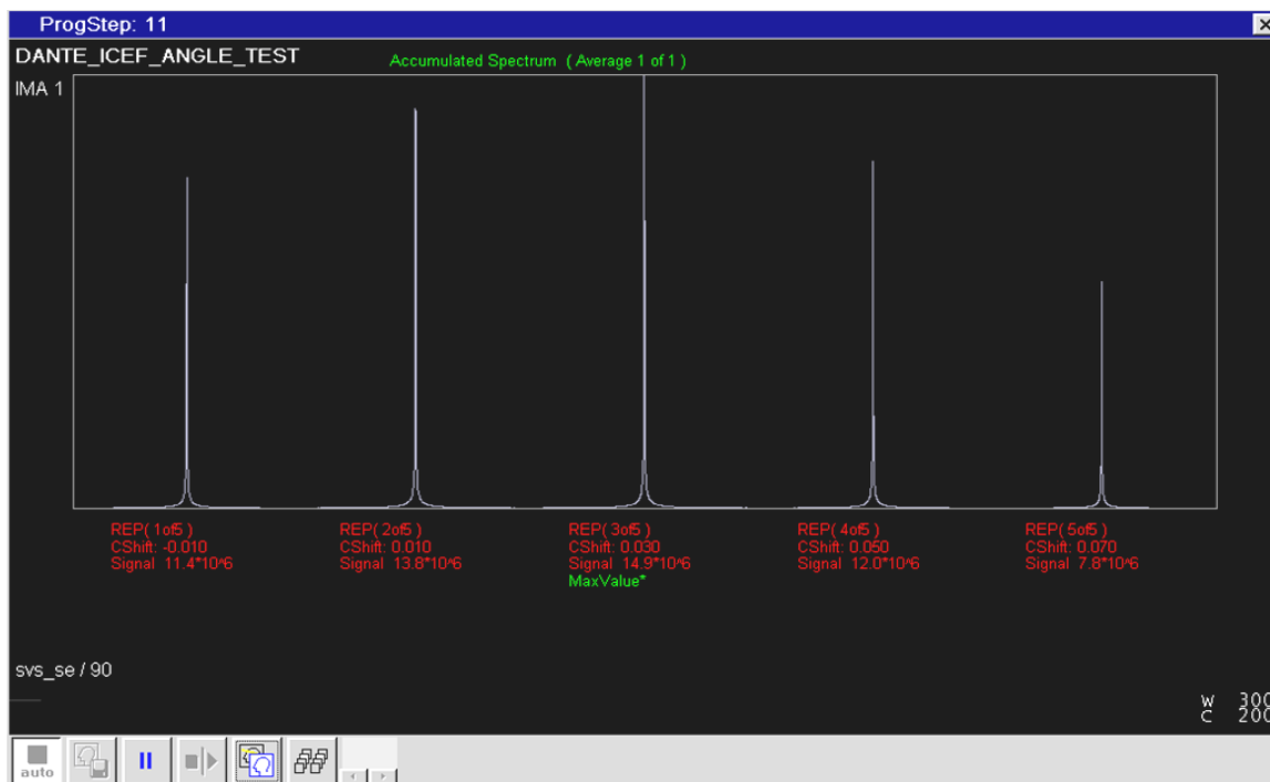
Figure C-6. The inline display illustrates the calibration of the DANTE chemical shift for the water peak and highlights the maximum value with a green label (MaxValue*).
